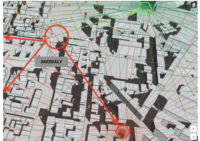
Fig.6. Spotting wrongfully connected UEs.
