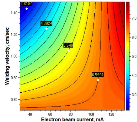
*Fig. 3. Contour plot of the mean values  $\tilde{y}_3$  of HAZ surface width depending on the variation of the electron beam current ( $p_1$ , mA) and the welding velocity ( $p_2$ , cm/sec) for a distance to the sample surface of  $z_3 = 295$  mm.*
