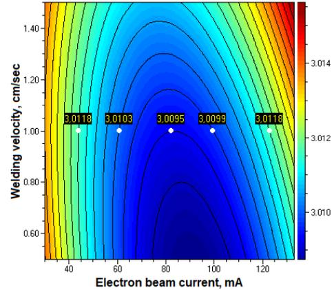
*Fig. 2. Contour plot of the standard deviations  $\tilde{s}_2$  of HAZ depth depending on the variation of the electron beam current ( $p_1$ , mA) and the welding velocity ( $p_2$ , cm/sec) for a distance to the sample surface of  $z_3 = 295$  mm.*
