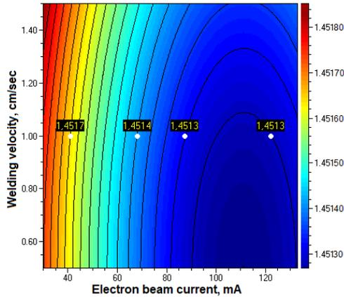
Fig. 4. Contour plot of the standard deviations  $\tilde{s}_3$  of HAZ surface width depending on the variation of the electron beam current ( $p_1$ , mA) and the welding velocity ( $p_2$ , cm/sec) for a distance to the sample surface of  $z_3 = 295$  mm.
