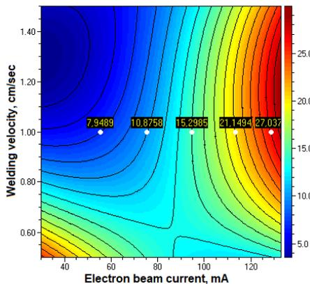
*Fig. 1. Contour plot of the mean values  $\tilde{y}_2$  of HAZ depth depending on the variation of the electron beam current ( $p_1$ , mA) and the welding velocity ( $p_2$ , cm/sec) for a distance to the sample surface of  $z_3 = 295$  mm.*
