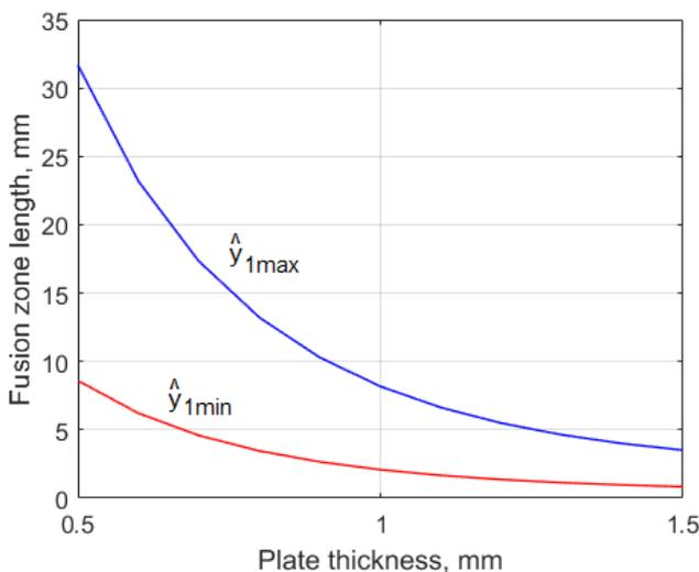
Fig. 3. Minimal fusion zone length  $\hat{y}_{1min}$  and maximal fusion zone length  $\hat{y}_{1max}$  depending on the plate thickness  $z_3$ .
