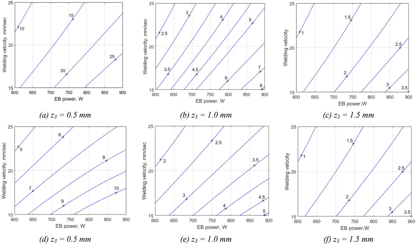
Fig. 1. Contour plots of the molten pool length  $\hat{y}_1$  (mm) along the  $x$ -axis (a, b, c), the molten pool width  $\hat{y}_2$  (mm) along the  $y$ -axis (d, e, f) as a function of the electron beam power  $z_1$  and the welding velocity  $z_2$  for different values of plate thicknesses  $z_3$ .
