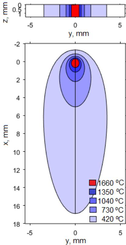
Fig. 2. Contour plots of the temperature distributions in x-y and y-z planes for electron beam power  $z_1 = 600$  W, welding velocity  $z_2 = 25.00$  mm/sec and plate thickness  $z_3 = 1.5$  mm and  $T_0 = 20$  °C
