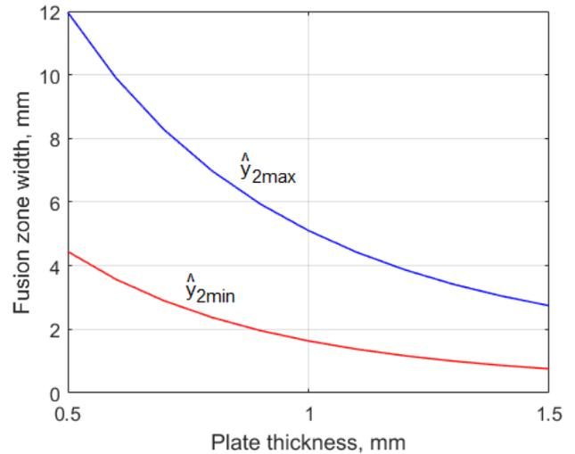
Fig. 4. Minimal fusion zone width  $\hat{y}_{2min}$  and maximal fusion zone width  $\hat{y}_{2max}$  depending on the plate thickness  $z_3$ .
