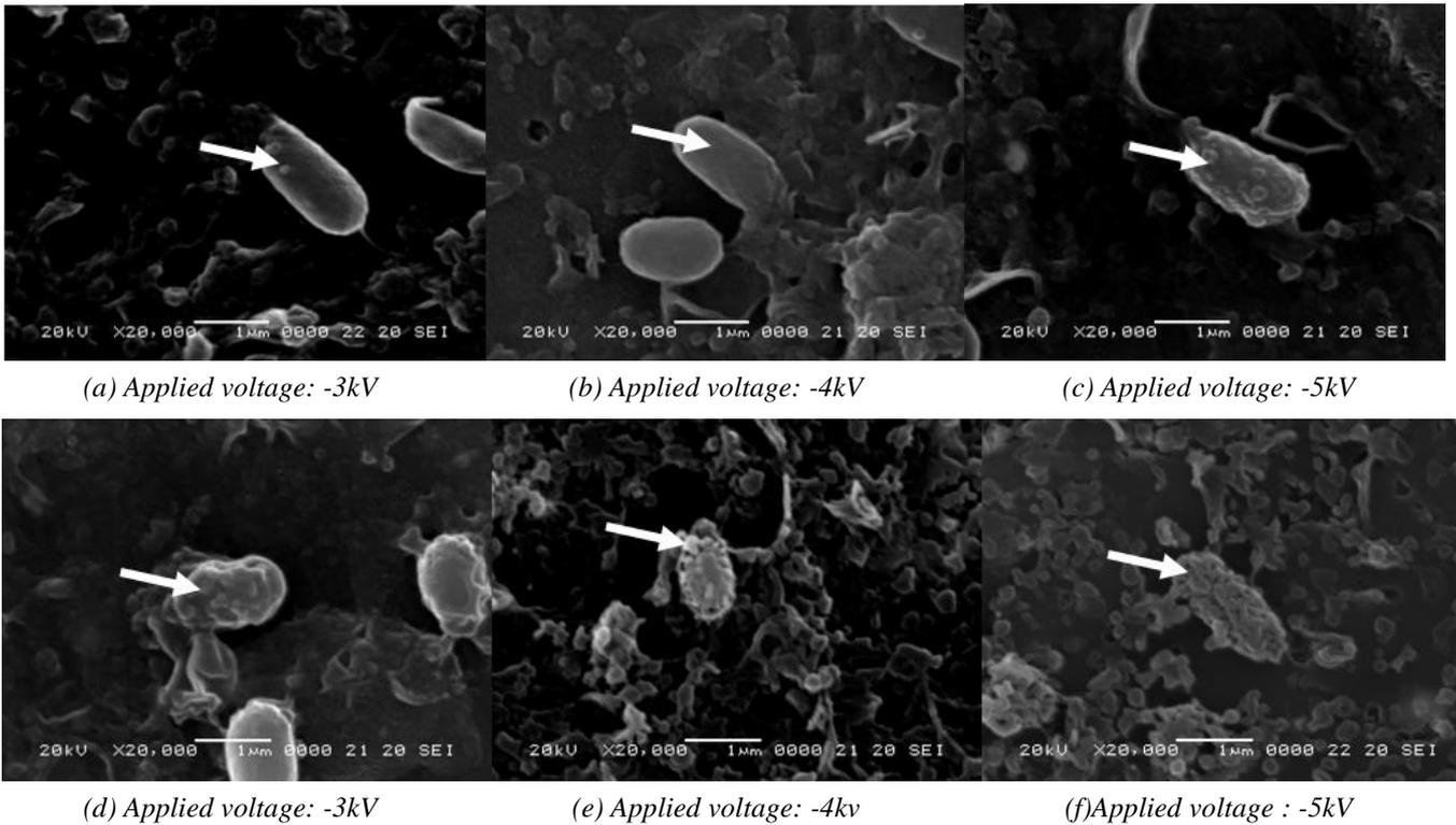
Fig.2. SEM photomicrographs of PBII-treated spores of *G. stearothermophilus* (a) – (c): Spores fixed on grass petri dish, (d)-(f): Spore fixed on stainless petri dish.
