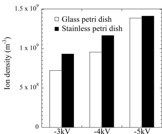
Fig.4. Relationship between petri dish material and ion density.
