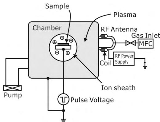
Fig.1. Schematic diagram of the PBII apparatus.
