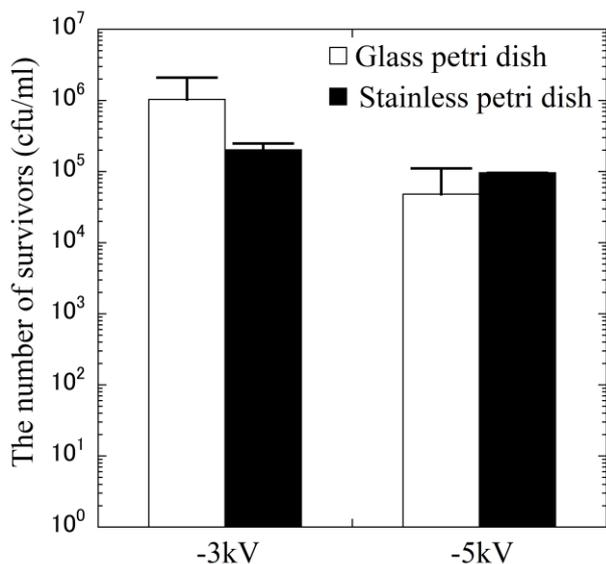
Fig.3. Influence of the material of petri dish on the sterilization effect.
