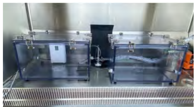
Fig.1. Experimental device for inactivating a new coronavirus using ozone [5].
