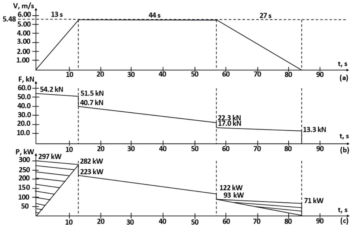
Fig. 2. Time diagrams: 2a: Time diagram of speed;
