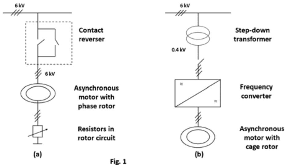
Fig. 1. 1a: Asynchronous motor with rheostat driving in phase rotor;
