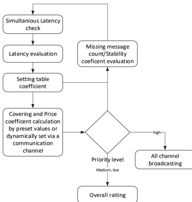
Fig.7. Flowchart of the algorithm for evaluating communication channels and their resilience.
