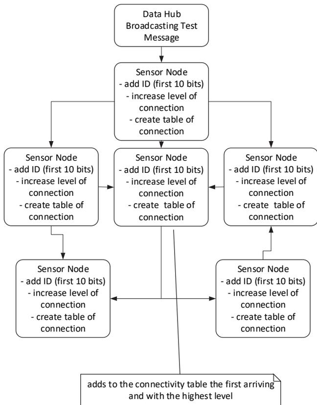
Fig.5. Connectivity table flowchart.
