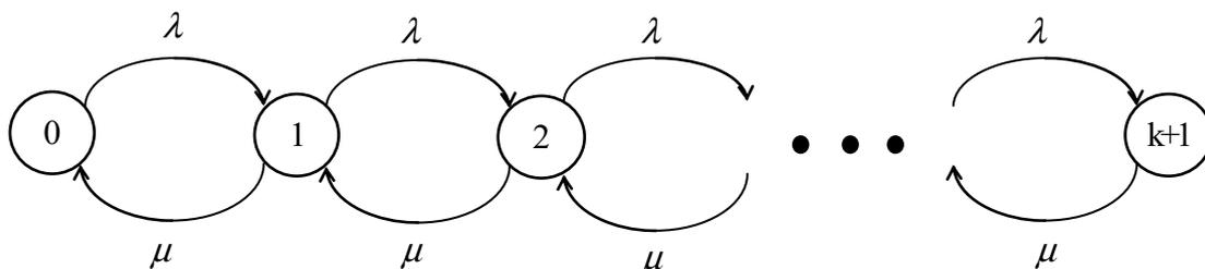
Fig.1. State transition diagram of the M/M/1/k system.
