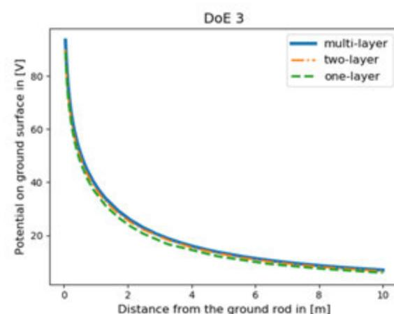
Fig.3. Comparison of the potential distribution on the ground surface for multi-layer soil and equivalent one/two-layer models for all used DoE – the rod length lower than one used in the optimization.
