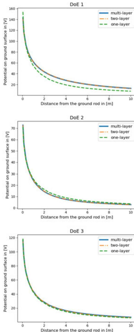
Fig.2. Comparison of the potential distribution on the ground surface for multi-layer soil and equivalent one/two-layer models for all used DoE – basic rod length.
