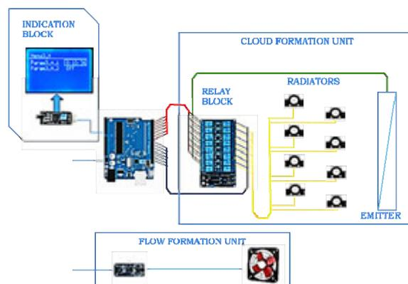
Fig. 3. Block diagram of the layout of the aromatic image synthesizer on the Arduino platform.
