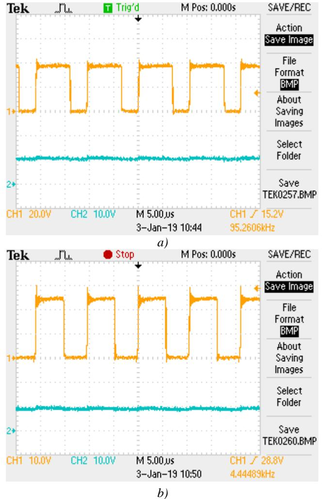
Fig.5. CH1 - drain-source voltage of VT2, CH2 - accumulator battery voltage, a) input voltage 20V, b) input voltage 13V
