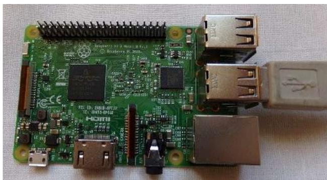
Fig. 6. The development platform “Raspberry Pi 3”.
