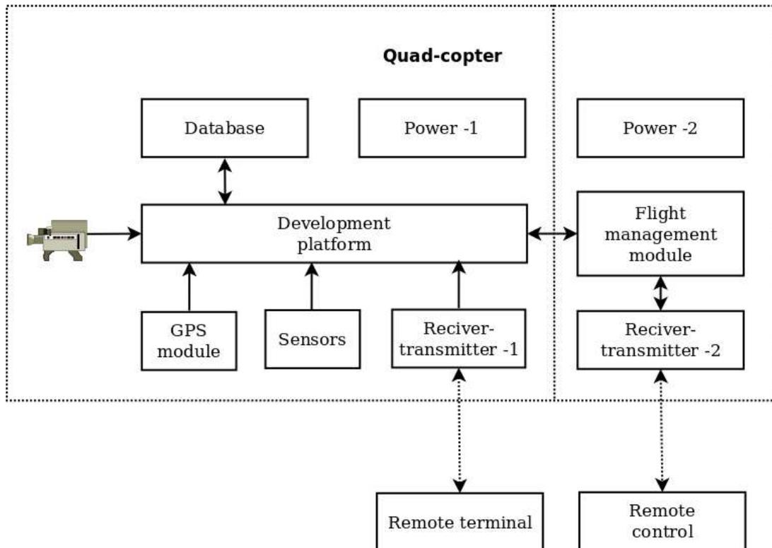
Fig.2. Architecture of the remote controlled system.
