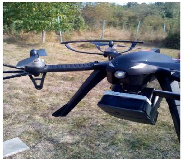
Fig.5. Attached development platform to quad-copter.
