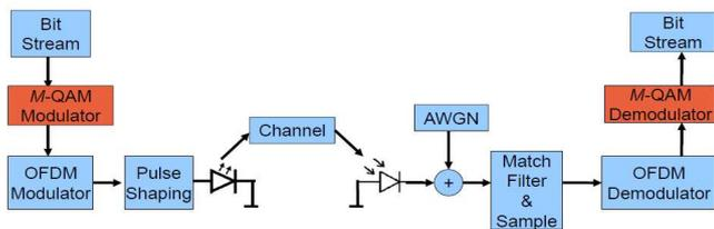
Fig. 4. A communication system based on OFDM.
