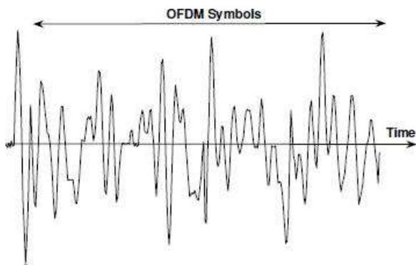
Fig. 5. Bipolar OFDM signal
