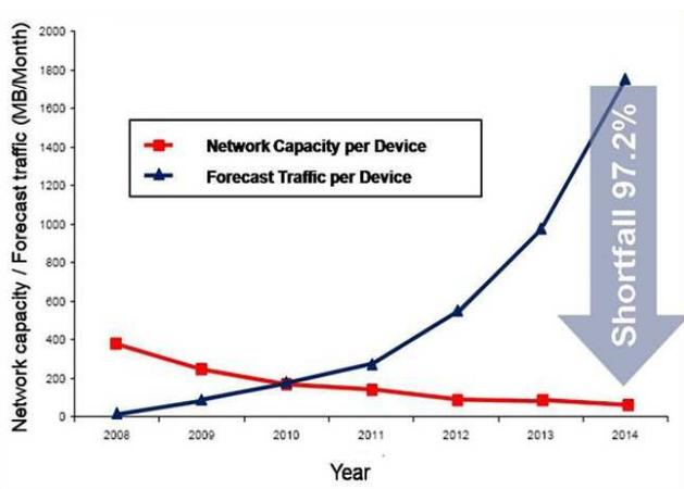
Fig. 2. The predicted, almost exponential, increase in demand of mobile communications services over the next years, and the corresponding network capacity evolution.
