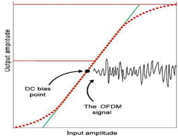
Fig. 6. Optical OFDM with DC bias DCO-OFDM
