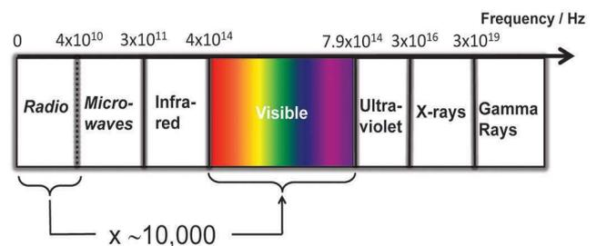
Fig.3. The electromagnetic spectrum and the vast potential of unused, unregulated, safe green spectrum in the visible light part. The visible light spectrum is 10,000 times larger than the entire radiofrequency spectrum.
