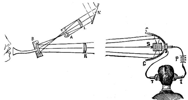
Fig. 1. The Photophone of Alexander Bell - transmitter and receiver
