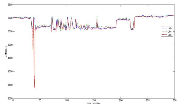
Fig. 2. Network voltage at PCC during EAF operating cycle.
