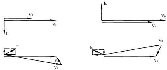
Fig. 6. Principle of power exchange in STATCOM.
