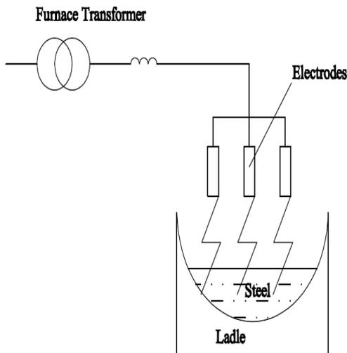
Fig. 1. Electric arc furnace structure.
