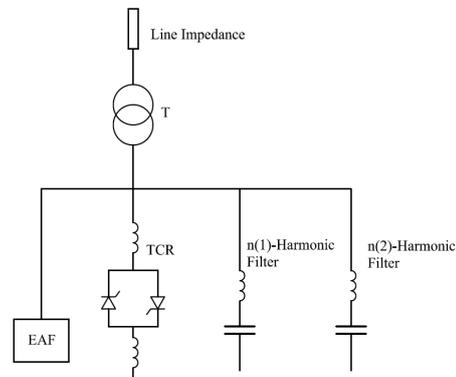
*Fig. 3. SVC typical single line diagram.*
