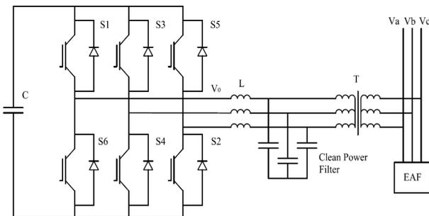
Fig. 5. STATCOM structure schema.
