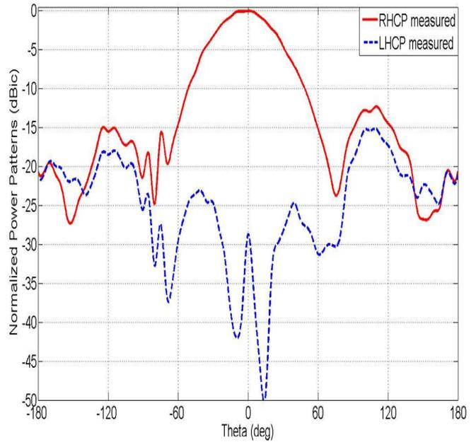
Fig.7. Measured  $\varphi = 45^\circ$  radiation pattern of a circularly polarized aperture coupled microstrip short backfire antenna at central frequency  $f_0 = 11.668$  GHz in the anechoic chamber: — copolarization (RHCP); - - - crosspolarization (LHCP).
