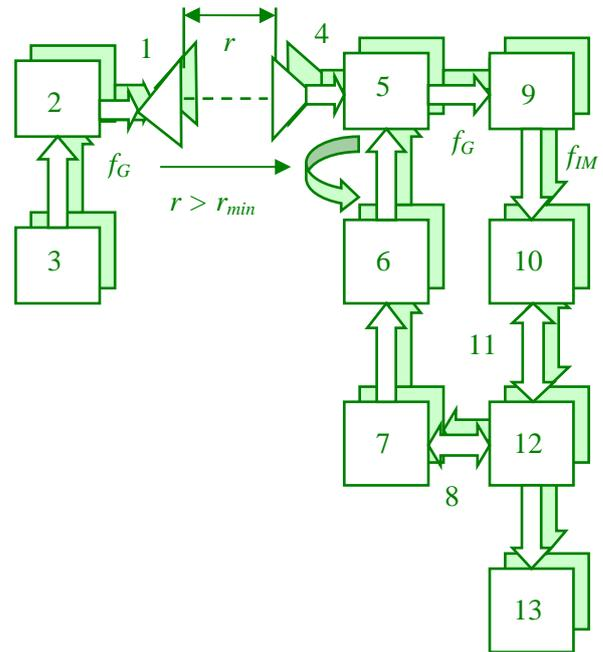
Fig.6. Block scheme of a system for automatic antenna measurements at frequency range 6-13 GHz with test receiver, spectrum analyzer and personal computer: 1 – transmitting antenna; 2, 5 – positioners; 3 – microwave generator; 4 – test antenna; 6 – DC motor; 7 – DC motor controller; 8, 11 – USB interfaces; 9 – test receiver; 10 – spectrum analyzer; 12 – personal computer, 13 – monitor.
