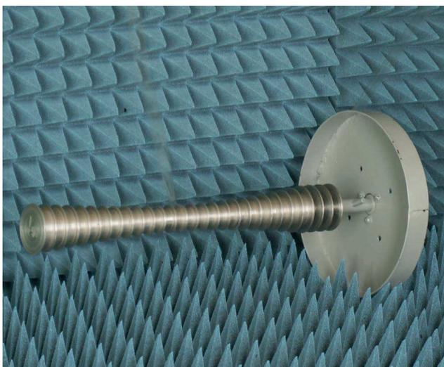
Fig.10. Impedance disk-on-rod antenna. BPO. Certificate of invention No. 26 928/12.07.1979.
