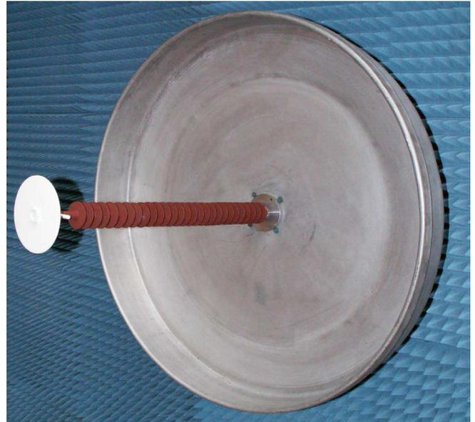
Fig.11. Backfire disk-on-rod antenna.
