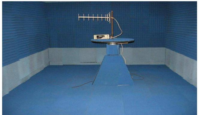
Fig.8. An anechoic chamber at TU-Varna.
