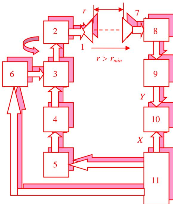
Fig.2. Block scheme of a system for automatic antenna measurements with test receiver and plotter: 1 – antenna under test; 2 – positioner; 3 – reducer; 4 – speed box; 5 – motor; 6 – microwave generator; 7 – receiving antenna; 8 – polarization positioner; 9 – test receiver; 10 – plotter; 11 – control panel.
