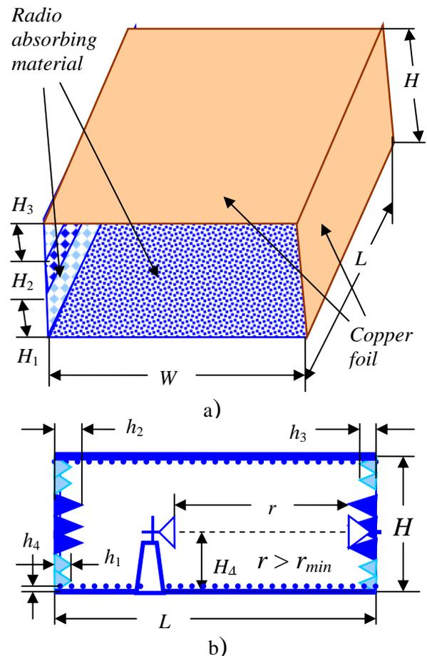
Fig.4. Geometry of an anechoic chamber for automatic antenna measurements: a) General view; b) Longitudinal section.
