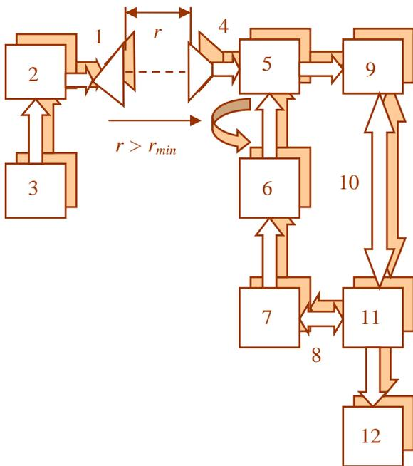
Fig.5. Block scheme of a system for automatic antenna measurements at frequency range 1-6 GHz with spectrum analyzer and personal computer: 1 – transmitting antenna; 2, 5 – positioners; 3 – microwave generator; 4 – test antenna; 6 – DC motor; 7 – DC motor controller; 8, 10 – USB interfaces; 9 – spectrum analyzer; 11 – personal computer; 12 – monitor.
