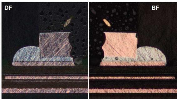
Fig.3. Specimen status after 6um polishing, dark field observation (left) and bright field observation (right).
