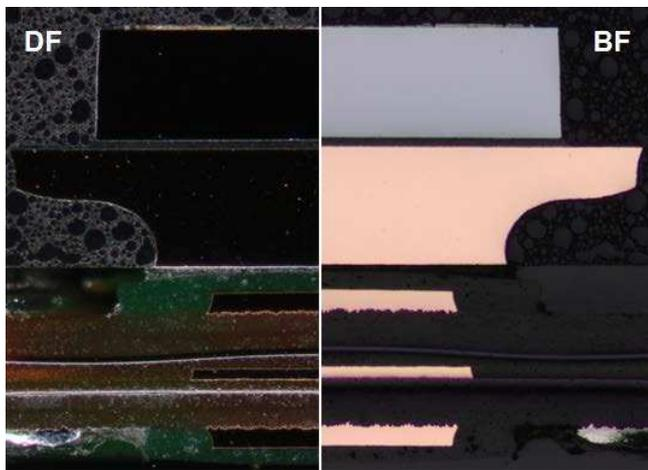
Fig.6. Specimen final status after 1um polishing, dark field observation(left) and bright field observation (right).
