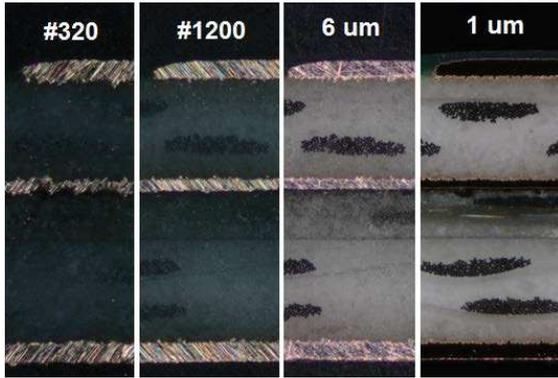
Fig.2. Specimen status at different process steps, dark field observation.
