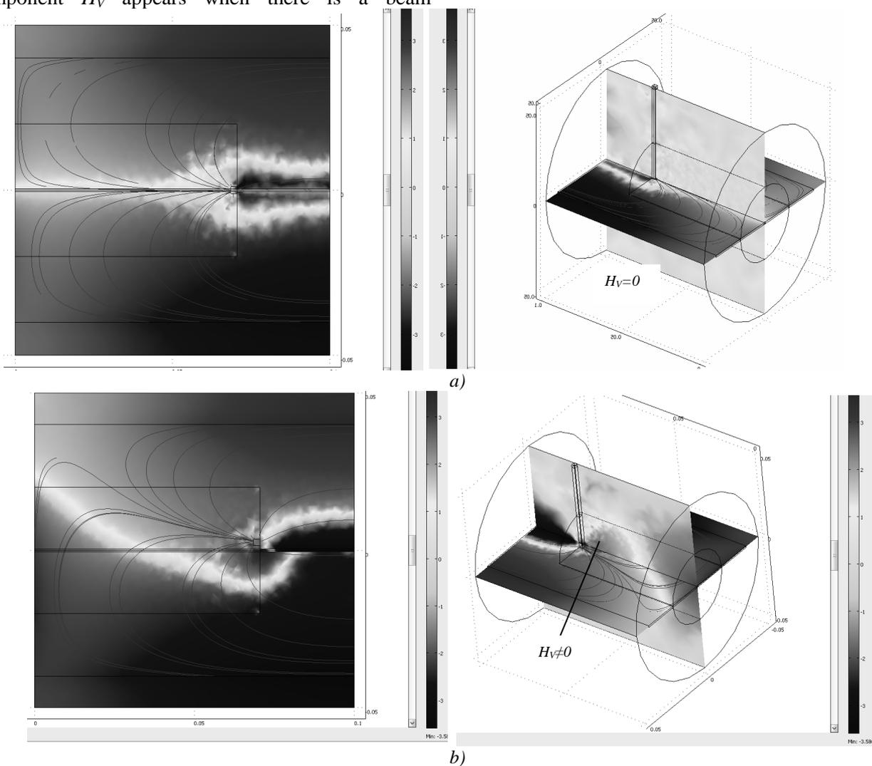
Fig. 2. Magnetic fields distribution: a –  $\varepsilon = 0$ ; b –  $\varepsilon = 0,1\text{mm}$  ( $\varepsilon$  – the beam deflection from the joint)
