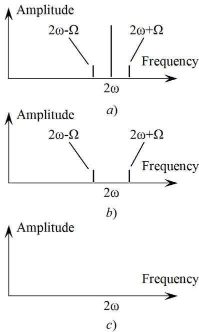
Fig. 4. Spectrum components of the Fluxgate measuring winding signal: a) -  $\varepsilon \neq 0$ ; Spectrum component of the measuring winding signal with uncompensated frequency  $2\omega$ ; b) -  $\varepsilon \neq 0$ ; Spectrum component of the measuring winding signal with compensated frequency  $2\omega$ ; c) -  $\varepsilon = 0$ ; spectrum component of the signal with frequency  $2\omega$  - compensated.
