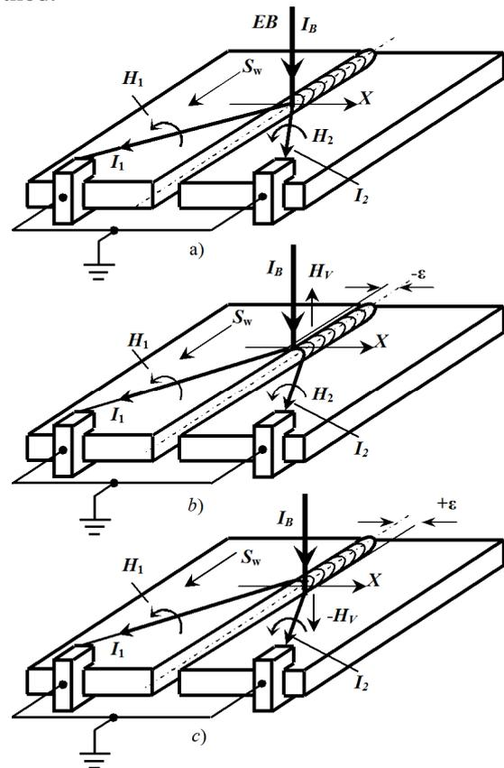
Fig.1. Dependence of the magnetic field vertical component on the electron beam position relative to: a) –  $X=\varepsilon=0$  (no displacement); b) –  $X=-\varepsilon$  (left displacement); c) –  $X=+\varepsilon$  (right displacement)
