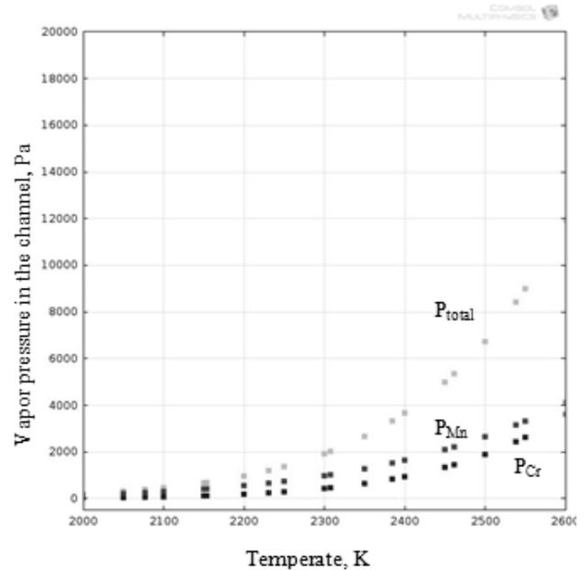
Fig. 2. Correlation between vapor pressure in the keyhole and the temperature for X12CrNiTi 18-10, where  $P_{Cr}$  is chrome vapor pressure;  $P_{Mn}$  is manganese vapor pressure;  $P_{total}$  – total vapor pressure.
