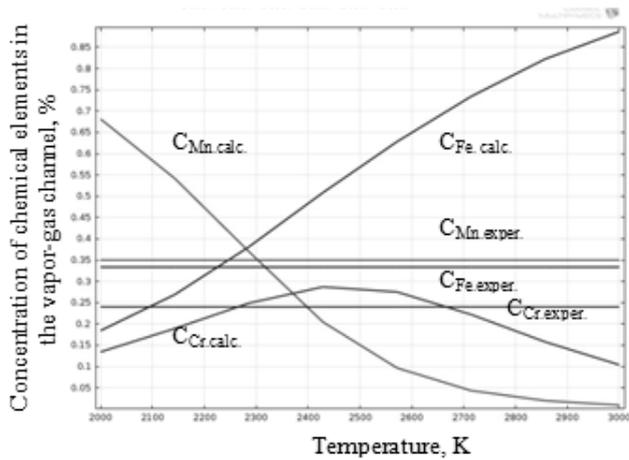
Fig.4. Correlation between iron, manganese and chrome concentrations in the channel for the X12CrNiTi 18-10 and the temperature
