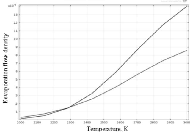
Fig.5. Evaporated element mass (Mn) in the channel for the X12CrNiTi 18-10 and the temperature
