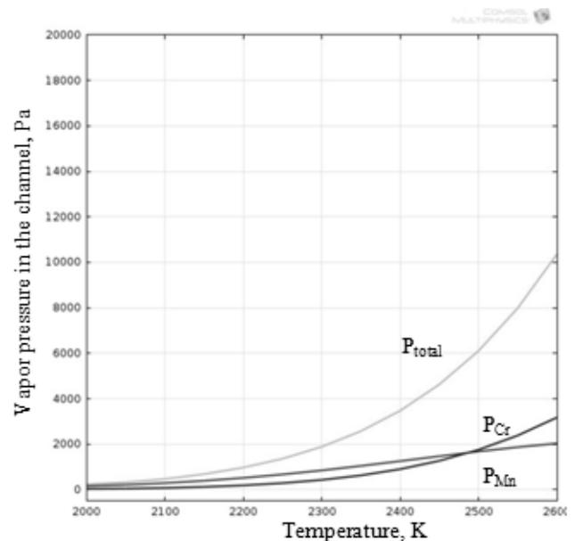
Fig. 3. Vapour pressure in the keyhole including the diffusion processes and the temperature for X12CrNiTi 18-10, where  $P_{Cr}$  is chrome vapor pressure;  $P_{Mn}$  is manganese vapor pressure;  $P_{total}$  – total vapor pressure
