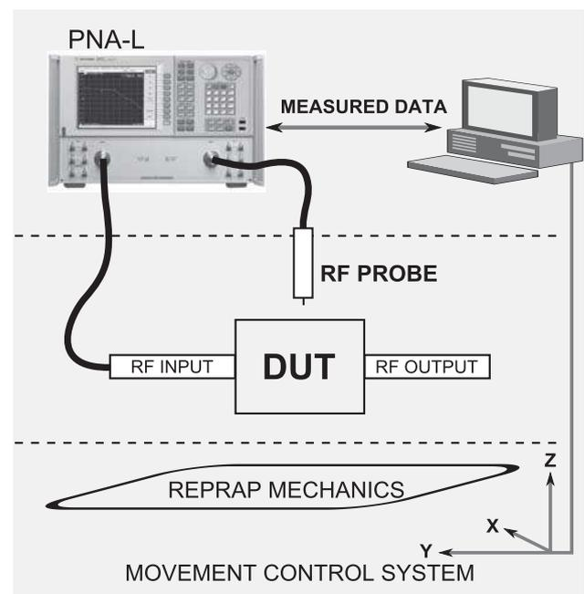
Fig.1. Simplified block diagram of near-field scanner.
