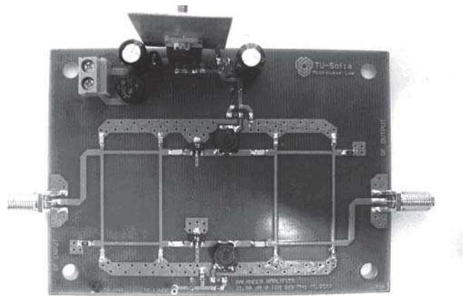
Fig.6. Balanced amplifier measured with the scanner.
