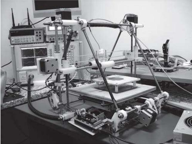
Fig.2. Photo of near-field measurement system.
