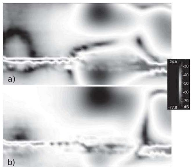
Fig.7. Surface currents amplitude for a) 760 b) 860 MHz.
