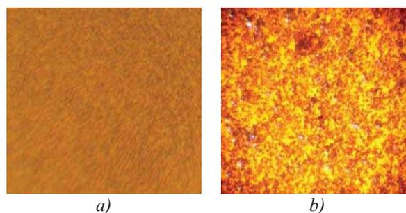
Fig. 1. Microscopic picture of the screen printed LMWC/polymer coating on ITO surface at magnification 100 a) treated with UV b) none treated with UV.
