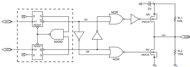
Fig. 3. An equivalent circuit of the PFD model.
