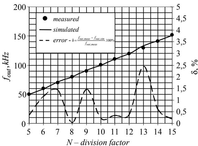
Fig. 7. Response data for the programmable frequency synthesizer.
