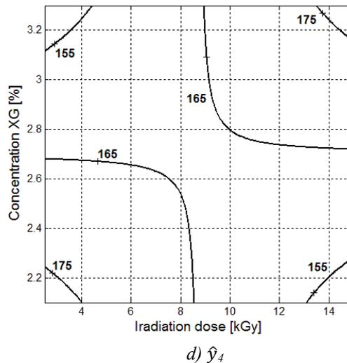
Fig. 2. Contour plots of the variation of a) gel fraction; b) swelling degree; c) elastic modulus and d) viscous modulus for constants: concentration of crosslinking agent  $z_2 = 1.25\%$  and concentration of CMC  $z_4 = 2.7\%$
