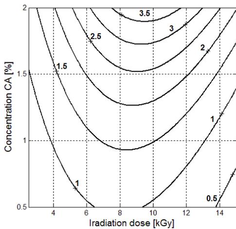
Fig. 1. Contour plot of the variance of the gel fraction  $s_1^2$
