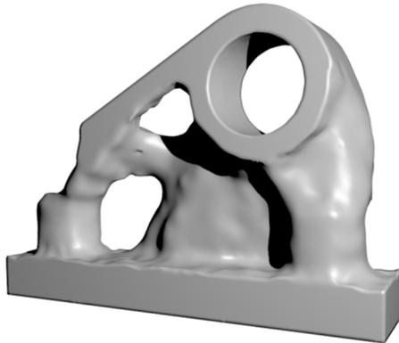
Fig. 1. Computer model of the bracket to be built by selective electron beam melting.
