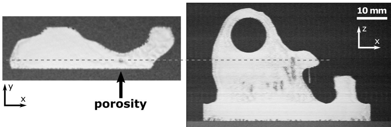
Fig. 2. Left: Electron optical (ELO) image acquired by backscatter electron detection. Depicted is the component cross-section at a height of ca. 20 mm. While most of the surface is smooth and dense, there is a single pore in the narrow part of the component. Right: Longitudinal cross-section through the 3D reconstruction of the component. It can be seen that the porosity seen in the 2D-ELO-image spreads across multiple layers.
