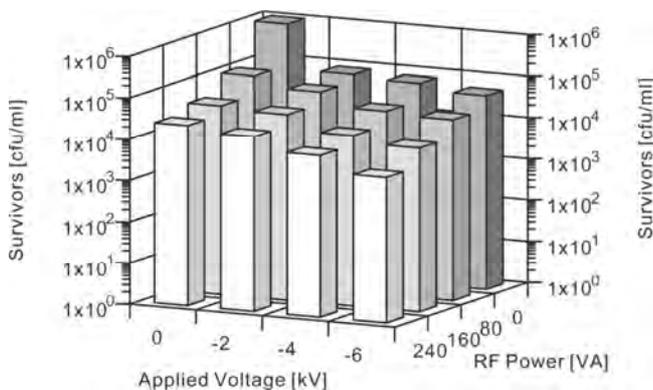
Fig.4. Result of sterilization treatment for *C. sporogenes* by PBII.
