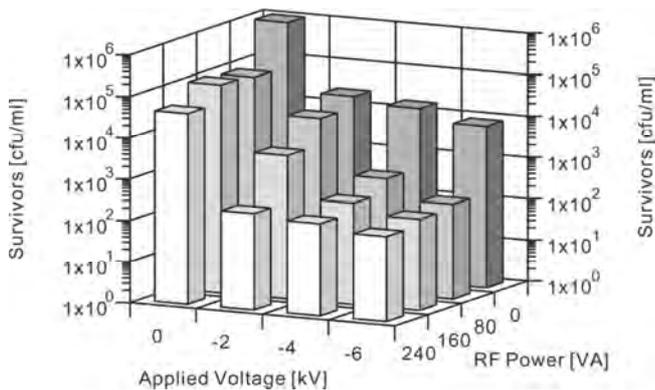
Fig.3. Result of sterilization treatment for *B. stearotherophilus* by PBII.
