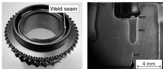
Fig. 1. Gear wheel with cross-section, weld depth 4 mm
