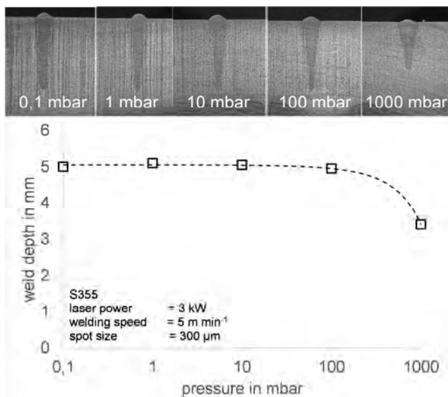
Fig. 6. Influence of the process pressure on the weld depth
