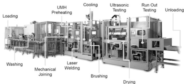
Fig. 9. Automated laser welding plant GEARline made by pro-beam.
