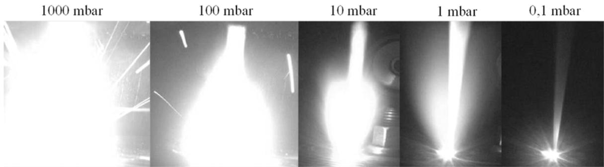
Fig. 3. Plasma plume at different pressure levels (laser power = 3 kW, welding speed = 50 mm s<sup>-1</sup>, spot size = 300 μm)
