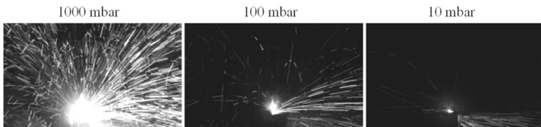
Fig. 4. Spatter formation at different pressure levels (source: ifs TU Brunswick)
