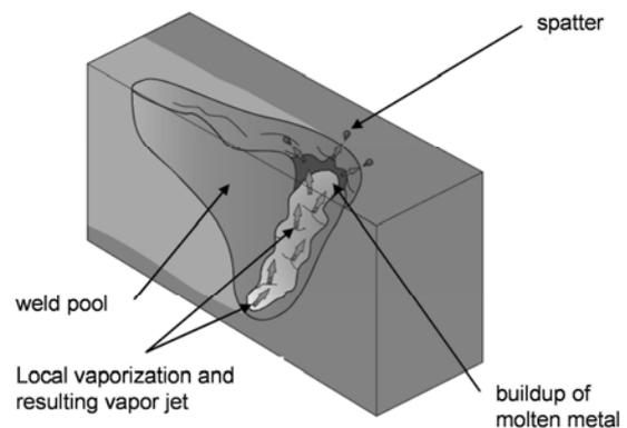
Fig. 5. Mechanism of spatter formation [10]
