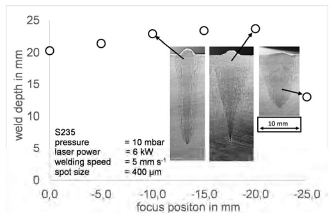
Fig. 7. Influence of the focus position on the weld depth
