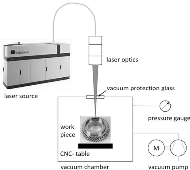
Fig. 2 Basic setup for laser beam welding under reduced pressure
