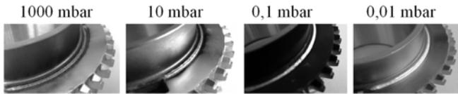
Fig. 8 Work piece contamination at different pressure levels
