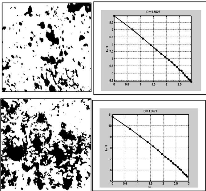
Fig. 3. Fractal analysis of the porous structure of the coating at different depths below the surface (the distance from the surface: top, 5  $\mu\text{m}$ ; bottom, 150  $\mu\text{m}$ ).
