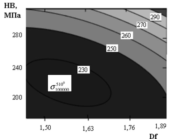
Fig. 4. Limit level lines long-term strength  $\sigma_{100000}^{510^{\circ}\text{C}}$  (MPa) for the weld metal 15H1M1F welded EBW in the coordinate field "Hardness-fractal dimension".
