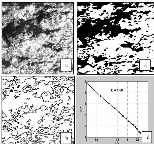
Fig. 2. Consecutive stages of processing the image of the initial fracture zone of the welded joint: (a) the actual image; (b), (c) the section of the fracture surface with the removed shadow and with the relief contour; (d) dependence of  $\ln P$  on  $\ln L$ , the fractal dimension of the fracture surface  $D = 1.68$ .
