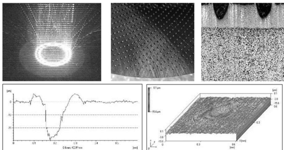
Fig.5. EB processing micro structures (cavities) and their topography
