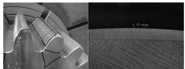
Fig. 3 left: Gear-wheel prototype EB hardened tooth flanks, right: Hardness increase zone (tooth cross section)
