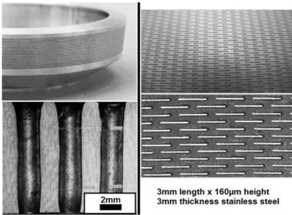
Fig. 3 top-left: Sieve food industry, bottom-left: drillings in 10mm material thickness, right: slot drilling in stainless steel
