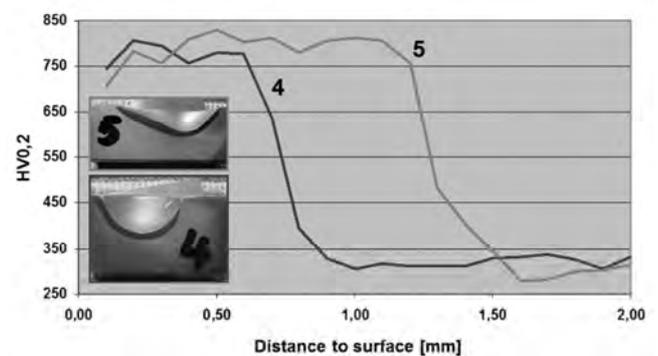
Fig. 2 Typical hardening depth on EB processed workpieces
