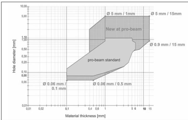
Fig.4. EB drilling spectrum (hole diameter vs material thickness) at pro-beam
