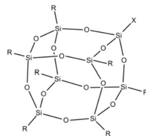
Fig. 1 Hydrogen Silsesquioxane (HSQ) molecule [2].
