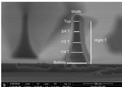
Fig.2. Measurement levels along the line height for the resist profiles in HSQ.
