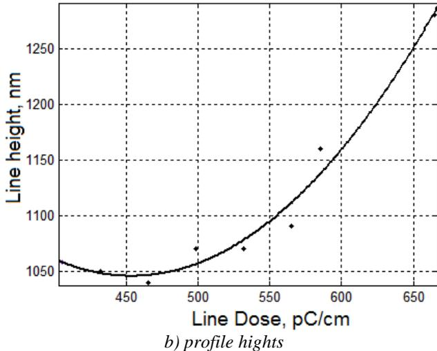
Fig. 5. Experimental and estimated dimensions of 1200 nm HSQ resist profiles (cross-sections)
