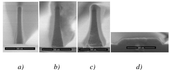
Fig.3. Comparison between resist profiles in 700 thick HSQ FOX-25 resist for various exposure line doses. The profile widths at the top/bottom levels of the resist thickness are: (a) 74 nm/115 nm for 555 pC/cm, (b) 90 nm/233 nm for 690 pC/cm, (c) 98 nm/410 nm for 863 pC/cm; (d) in 150 nm thin HSQ - 635 nm/857 nm for 1021 pC/cm
