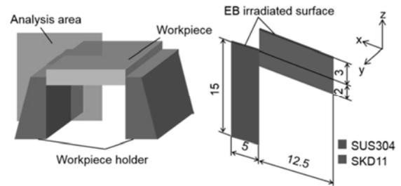
Fig. 7. Heat conduction analysis model
