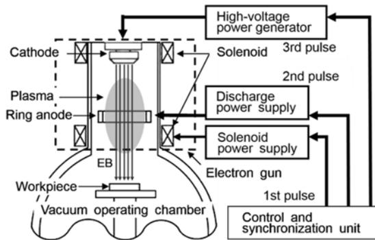
Fig.3. Large-area EB irradiation equipment
