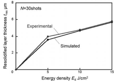
Fig.10. Comparison of simulated resolidified layer with experimental one
