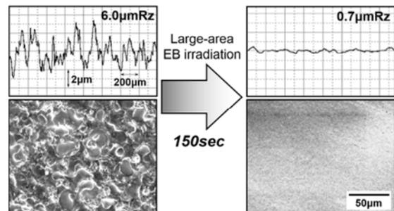
Fig.1. Surface roughness curves and SEM images of surface before and after EB irradiation.
