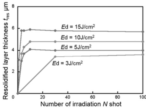
Fig. 6. Variations of resolidified layer thickness
