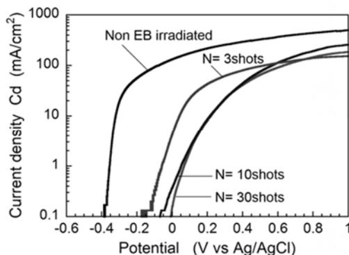
Fig.12. Anodic polarization current density of large-area EB irradiated surfaces.
