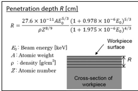
Fig.8. Consideration of electron penetration effect
