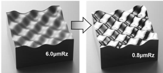
Fig.2. Large-area EB irradiated sample.
