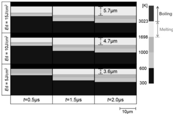
Fig.9. Simulated temperature distributions at workpiece surface
