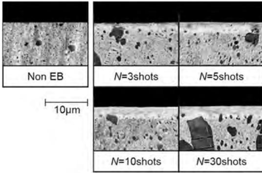
Fig. 5. Cross-sectional SEM images of resolidified layer with different EB irradiation number
