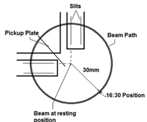
Fig. 3. Beam scanning over the probe. (Reproduced by permission of TWI Ltd.)
