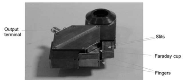
Fig. 2. Construction of the probe. (Reproduced by permission of TWI Ltd.)
