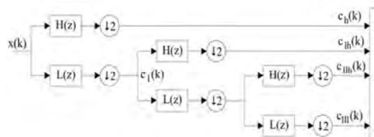
Fig. 5. Decomposition of signal to 3 levels. [9]
