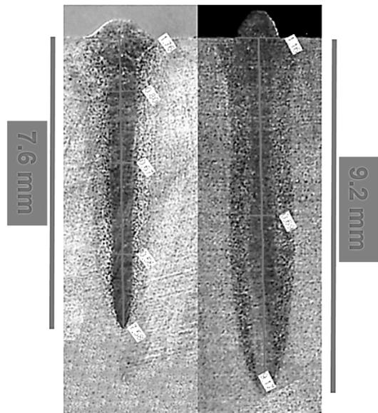
Fig. 6. Cross section of two EB welds with 3 kW beam power and different surface spot size
