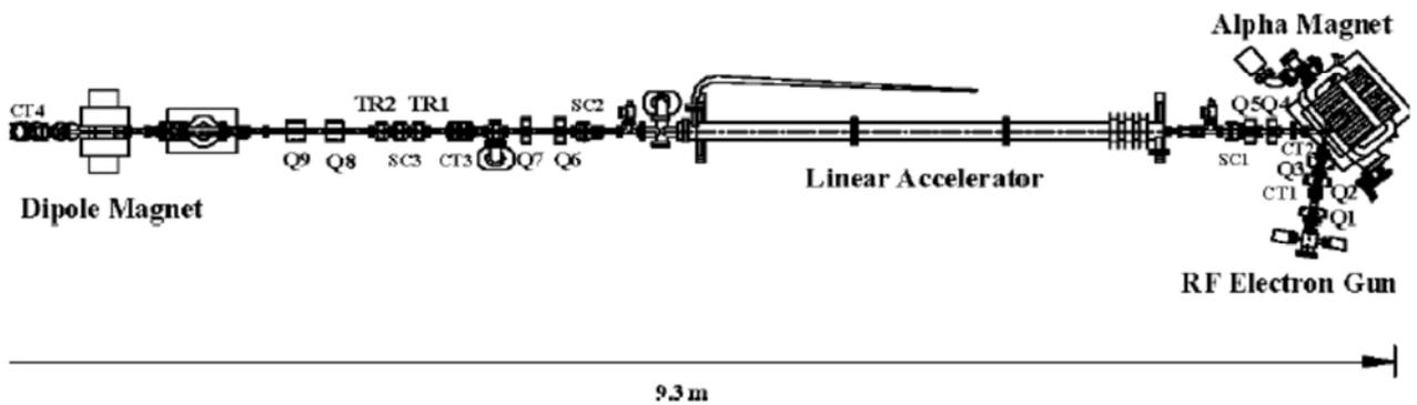
Fig. 1. SURIYA facility. Upper: photo. Lower: schematic diagram of the layout of the SURIYA electron linac and beamline system at Chiang Mai University. Q: quadrupole magnet. CT: current monitor. SC: screen monitor. TR: transition X-radiation experimental station. PXR: parametric X-radiation experimental station.
