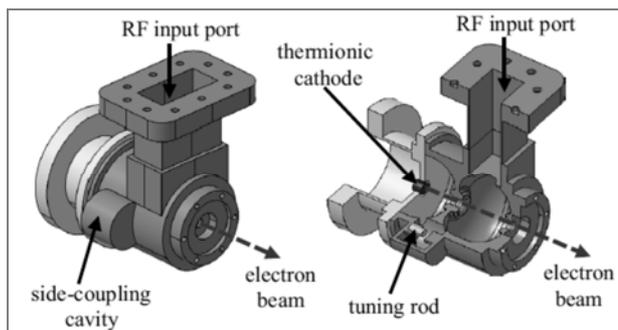
Fig. 2. Schematic diagram in 3D and cut-view of the side-coupling thermionic RF gun of the SURIYA facility.
