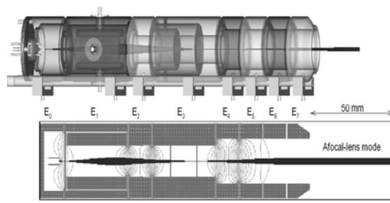
Fig. 3. 3D-AutoCAD view of the electron gun used in the electron trajectories simulations.
