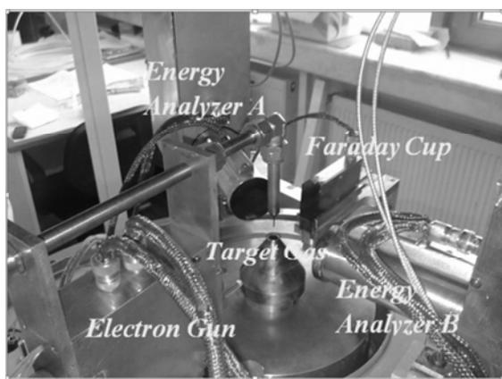
Fig. 2. A photo of the interaction region in the experimental system.
