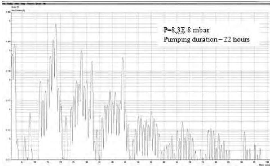
Fig. 4. Spectrum of test vacuum system with a testing chamber.
