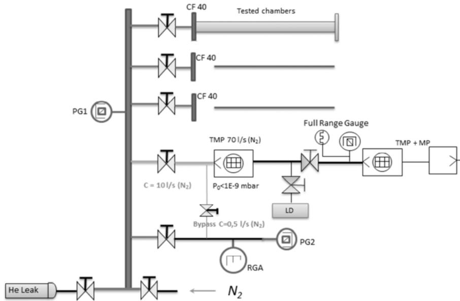
Fig.3. The setup for vacuum tests (PG1, PG2 – penning gauges, RGA – residual gas analyzer, TMP – turbo-molecular pump, MP – mechanical oil-free pump, LD – leak detector (sensitivity better than  $1E-10 \text{ l} \cdot \text{mbar/s}$ ), He leak – stable, known He leak)
