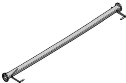
Fig. 1. The bended chamber with fixation to magnet
