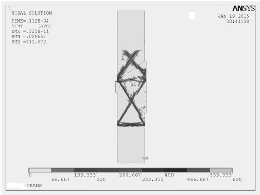
Fig.2. Nature of change of intensity of tension in a pipe wall on border metal seam in  $t \approx 0.111 \cdot 10^{-4}$  sec time-point
