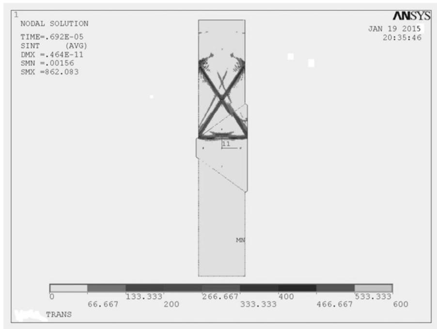
Fig.1. Nature of change of intensity of tension in a pipe wall on border metal seam in  $t \approx 0.629 \cdot 10^{-5}$  sec time-point
