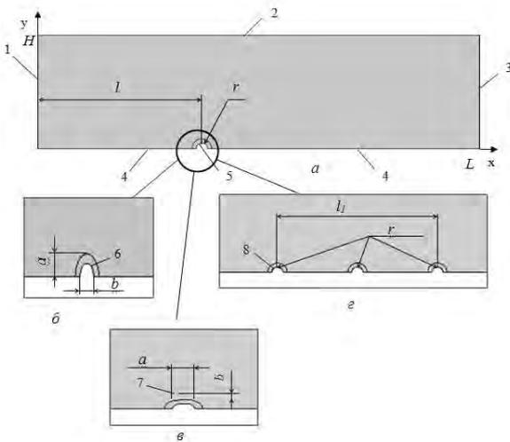
Fig.1. Calculated geometry of the problem: a - static beam; б, в - longitudinal and transverse oscillation of the electron beam; z - a dynamic splitting of the electron beam on the three thermal power.
