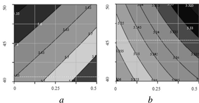
Fig.6. Influence of parameters of welding conditions to change the concentration of magnesium in the joint: a) Y axis – beam current, x axis – amplitude of beam oscillations b) X axis welding speed; Y-axis - the amplitude of the oscillations along
