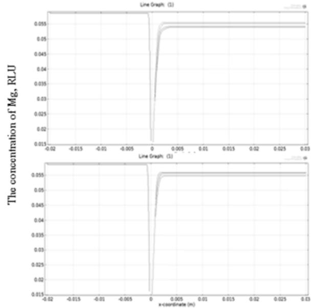
Fig.2. The results of numerical modeling of the magnesium content in the seam when oscillations of the electron beam
