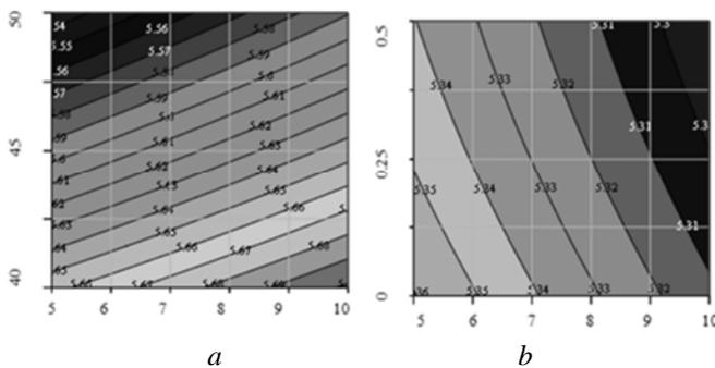
Fig.5. Influence of parameters of welding conditions to change the concentration of magnesium in the joint: a - the X axis welding speed Y-axis - the amplitude of the oscillations along; b - Y-axis - the amplitude of the oscillations along the x axis - welding speed
