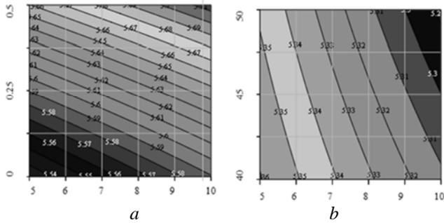
Fig.4. Influence of parameters of welding conditions to change the concentration of magnesium in the joint: a - Y-axis - the amplitude of the oscillations along the X axis - welding speed; b - along Y axis - the beam current, on the X axis - the welding speed
