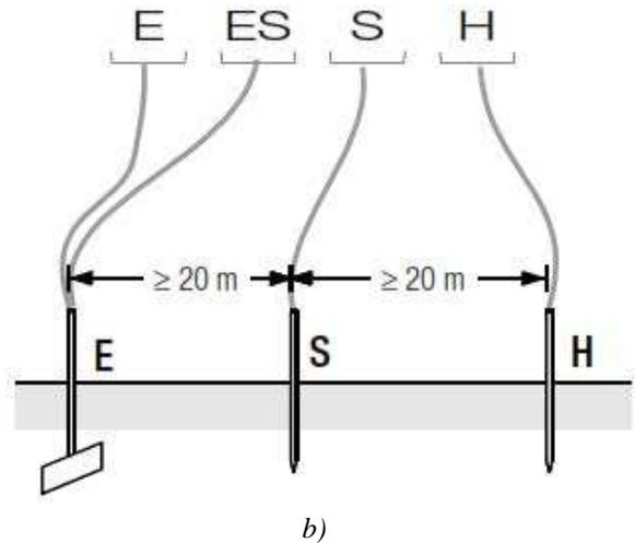
Fig.4. Measuring earthling resistance with a) Three wire test setup; b) Four wire test setup.
