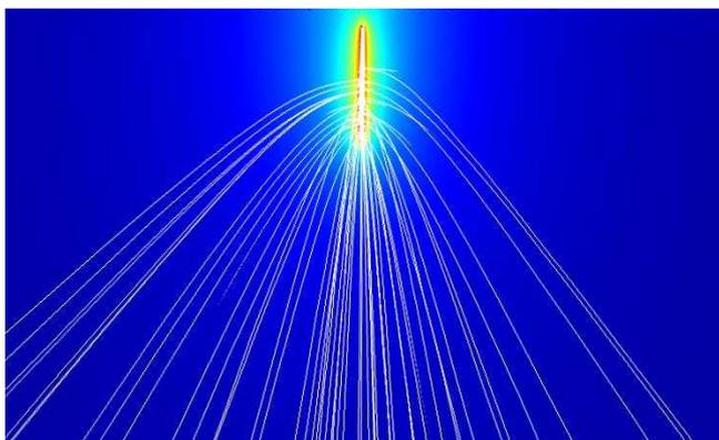
*Fig.6. Current and potential distribution of vertical rod electrode.*
