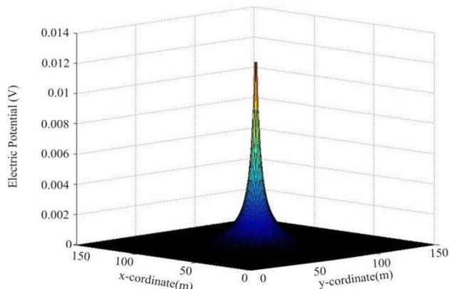
*Fig.8. The potential distribution at the ground surface of vertical rod electrode.*
