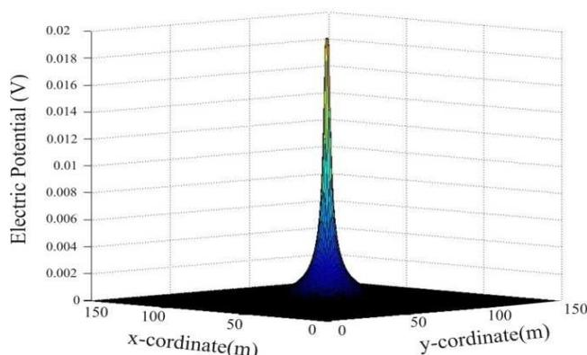
*Fig.9. The potential distribution at the ground surface of horizontal rod electrode,*
