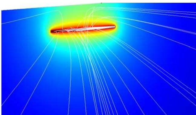
*Fig.7 Current and potential distribution of horizontal rod electrode.*
