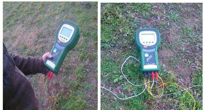
Fig.5. Experimental measuring of rod electrode resistance.
