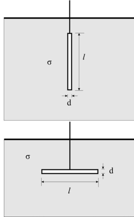
Fig.2. Vertical and horizontal ground rod electrode.
