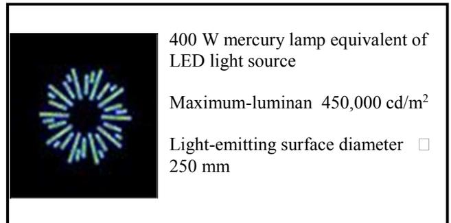
Fig. 2. Test target light source.
