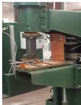
Fig.1. The spot resistance welding machine.
