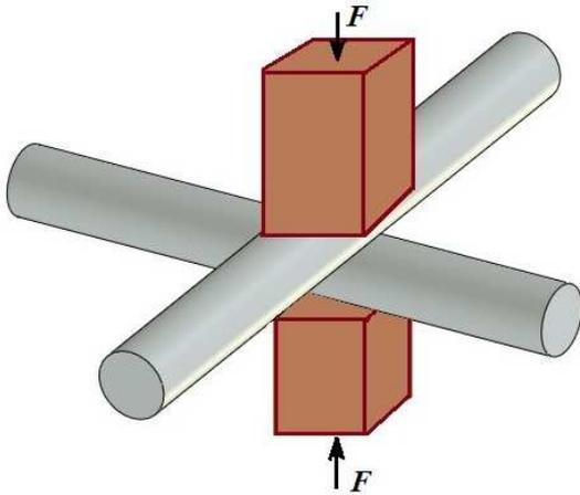
Fig.2. Illustration of spot resistance welding of crossed cylinders.
