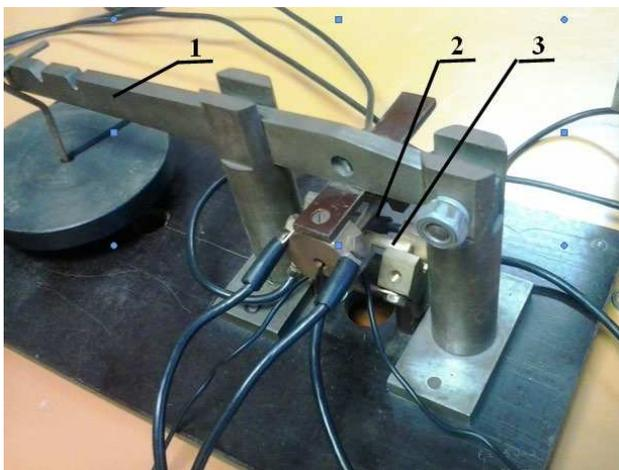
Fig.3. The mechanical part of the experimental set for the contact resistance measurement.
