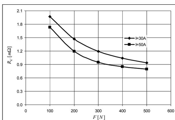
*Fig.10. Relationship between the average value of the contact resistance and the contact pressure force – untouched samples (d=10 mm).*
