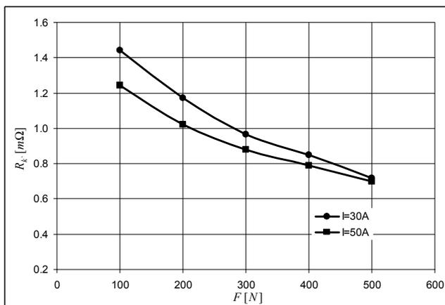
*Fig. 7. Relationship between the average value of the contact resistance and the contact pressure force – conditioned samples (d=6 mm).*
