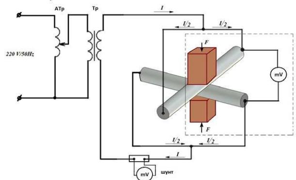
Fig.5. Electrical scheme used for the contact resistance measurement.
