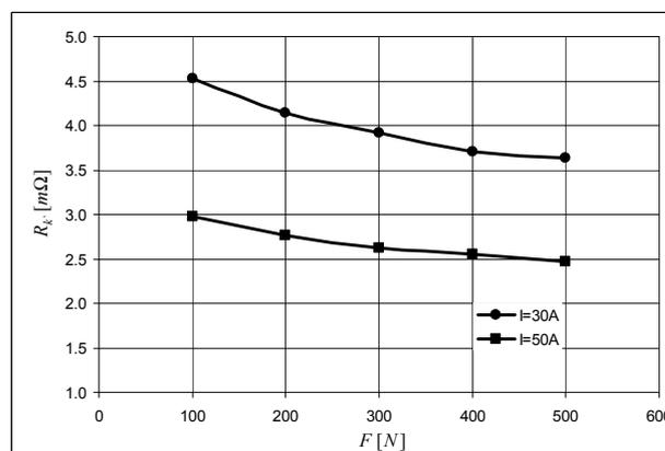
*Fig. 8. Relationship between the average value of the contact resistance and the contact pressure force – untouched samples (d=8 mm).*
