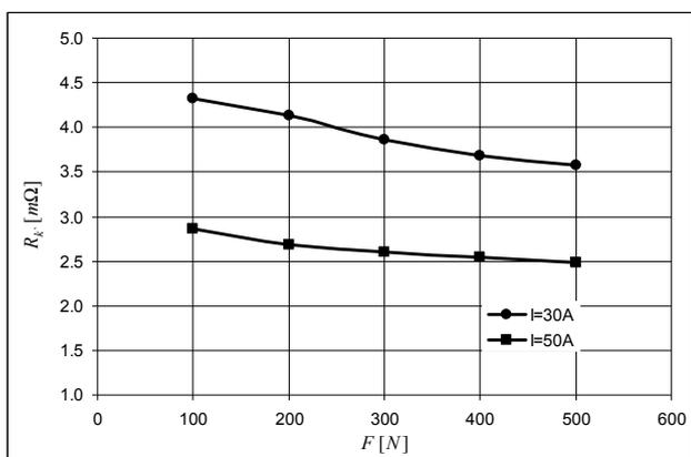
*Fig. 6. Relationship between the average value of the contact resistance and the contact pressure force – untouched samples (d=6 mm).*
