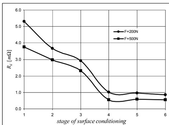
Fig.12. The average value of the contact resistance versus selected six degrees of surface conditioning.
