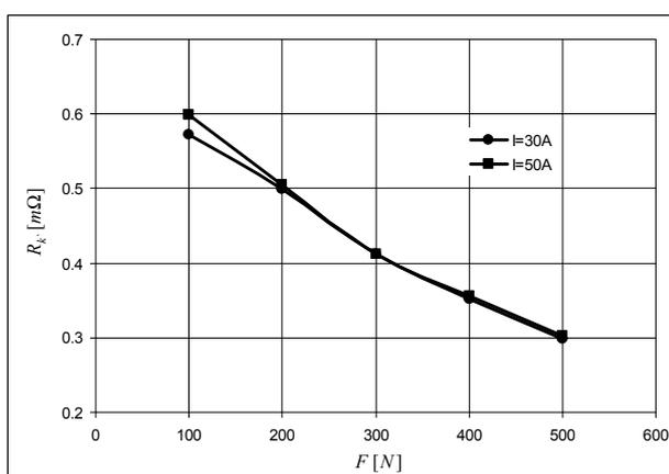
*Fig.11. Relationship between the average value of the contact resistance and the contact pressure force – conditioned samples (d=10 mm).*
