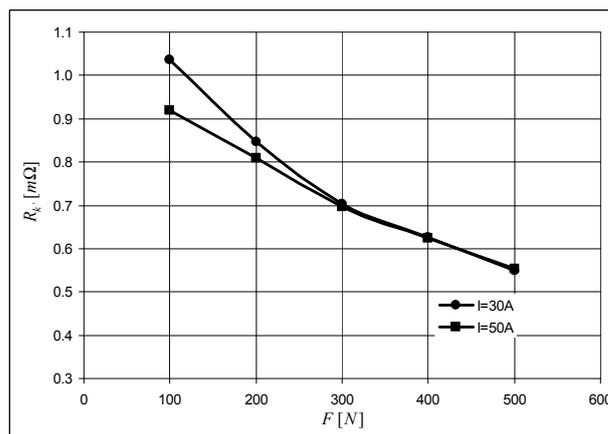
*Fig. 9. Relationship between the average value of the contact resistance and the contact pressure force – conditioned samples (d=8 mm).*
