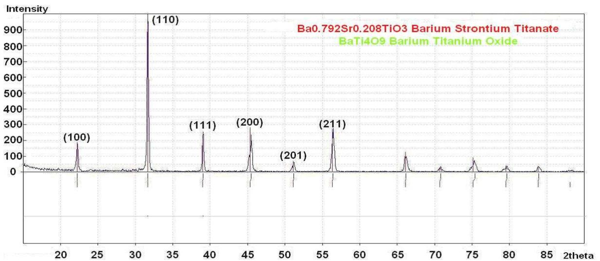
Fig.2. X-ray diffractogram of composition  $Ba_{0.8}Sr_{0.2}TiO_3$  at temperature of synthesis  $1150^{\circ}C$ .
