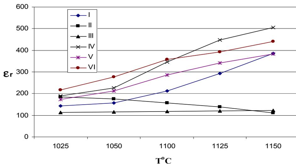
*Fig.4. Dependence of the relative permittivity on the temperature of synthesis.*
