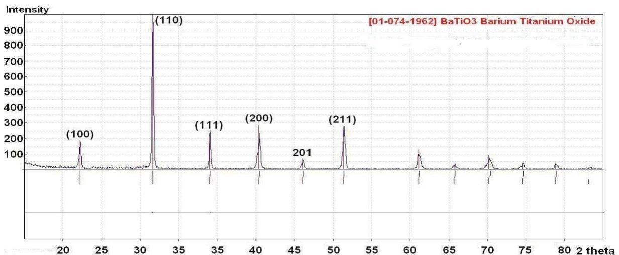
Fig. 1. X-ray diffractogram of composition Ba<sub>0,9</sub>Sr<sub>0,1</sub> TiO<sub>3</sub> at temperature of synthesis 1150°C.
