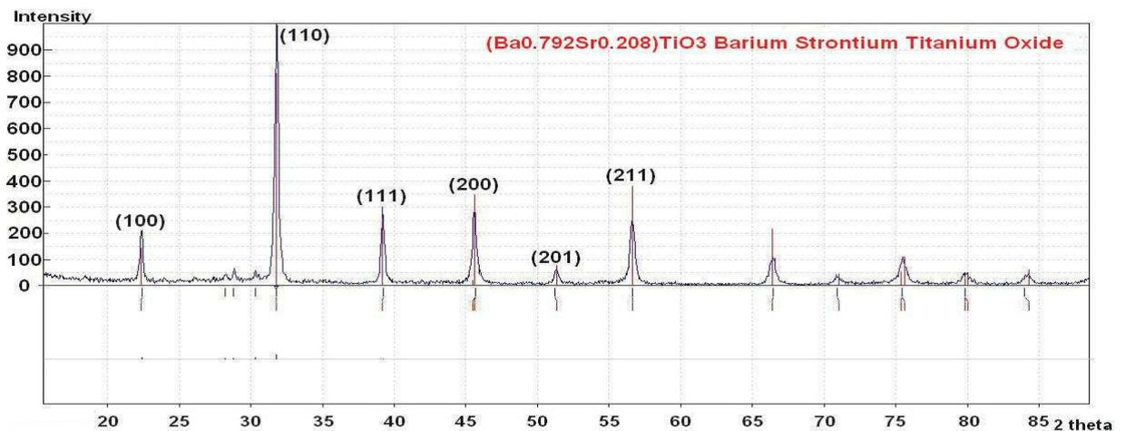
Fig.3. X-ray diffractogram of composition  $Ba_{0.8}Sr_{0.2}TiO_3 + 5wt\% H_3BO_3 + 15wt\% Bi_2O_3$  at temperature of synthesis  $1150^{\circ}C$ .
