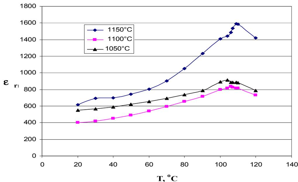
Fig.5. Dependence of the relative permittivity on the temperature of composition  $Ba_{0.8}Sr_{0.2}TiO_3 + 5wt\% H_3BO_3$ .
