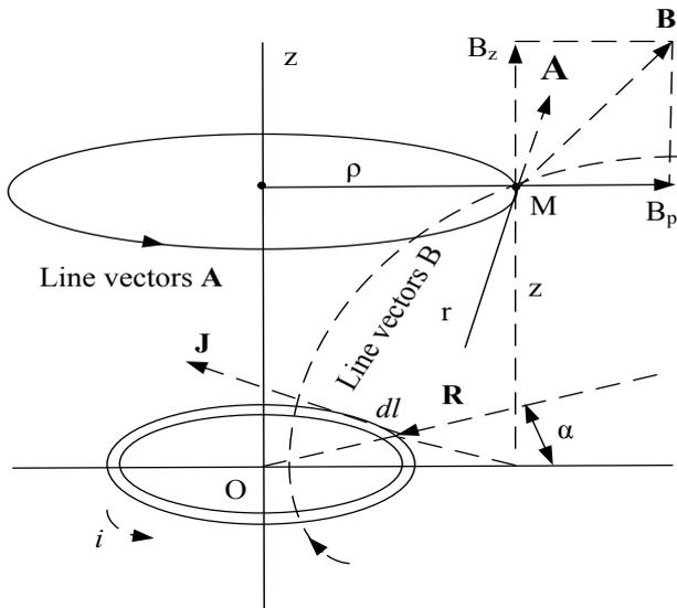
Fig.1. Field of circular contour.
