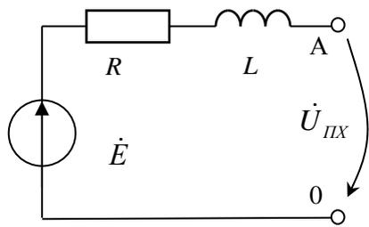
Fig. 4. Equivalent electric circuit at idle running.
