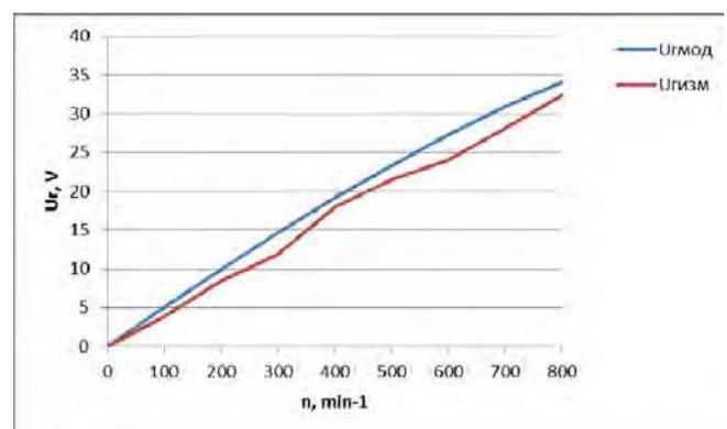
Fig. 7. Phase voltages of both the model and the generator at active load.
