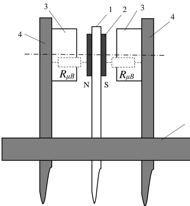
Fig. 1. Constructive scheme of the two-section generator and a view from the left
