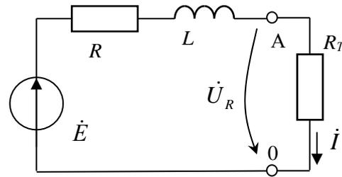
Fig. 6. Equivalent electric circuit at active load.
