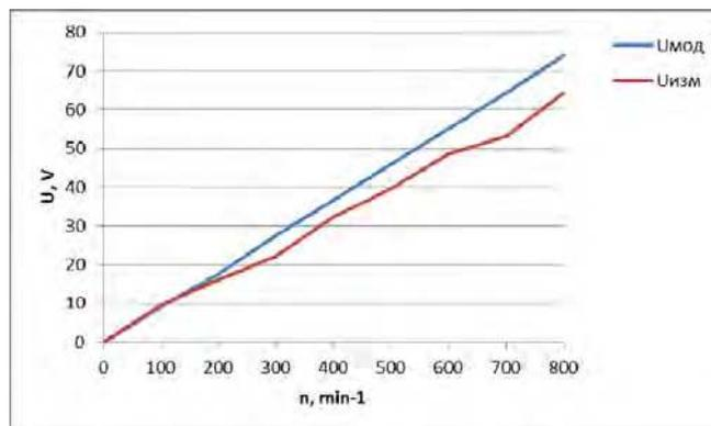
Fig. 5. Phase voltages of both the model and the generator at idle running.
