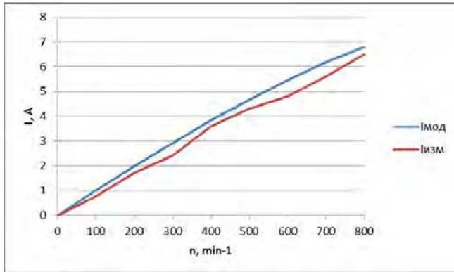
Fig. 8. Phase currents of both the model and the generator at active load.
