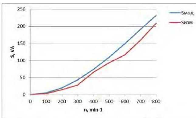
Fig. 9. Phase full power of both the model and the generator at active load.
