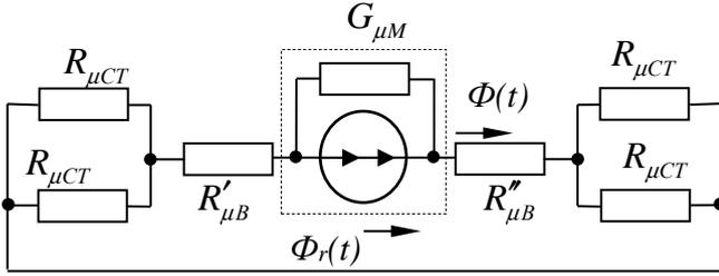
Fig. 3. Equivalent magnetic circuit
