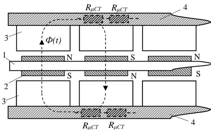
Fig. 2. Constructive scheme of part of the generator, a top view
