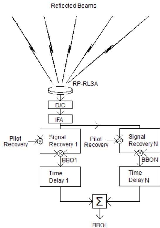
Fig. 6. Block-scheme of SCP Rake receiver in HAPS mixed LOS and NLOS propagation environment.
