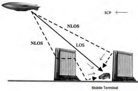
Fig. 5. Possible use of SCP-RPSC technology in HAPS mixed LOS and NLOS propagation environment
