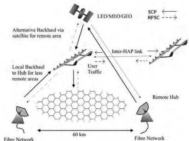
Fig. 4. Possible use of SCP-RPSC technology in HAPS feeder lines and inter HAPS links.
