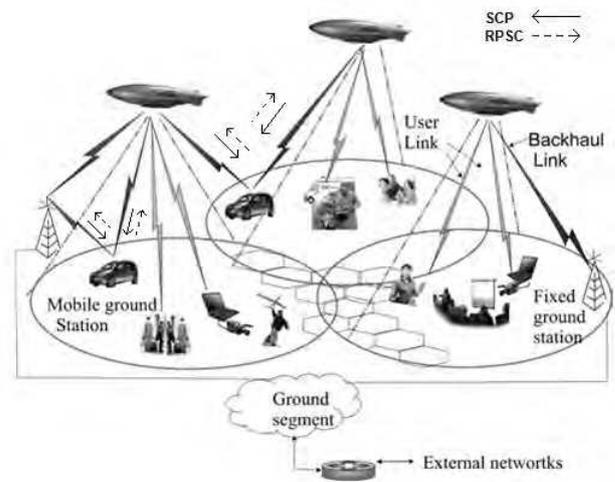
Fig.3. Possible applications of SCP-RPSC technology in HAPS LOS terminals.
