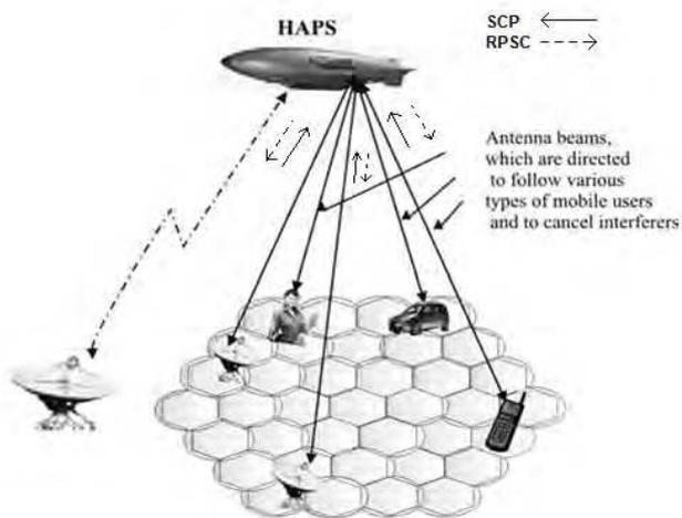
Fig.2. Architecture of a SCP-RPSC HAPS base station.
