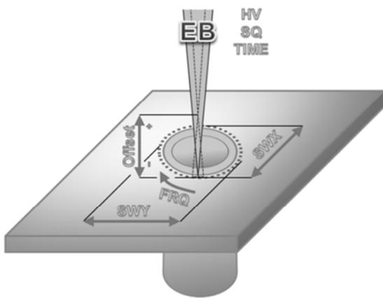
Fig.1. Flash electron beam welding parameters scheme
