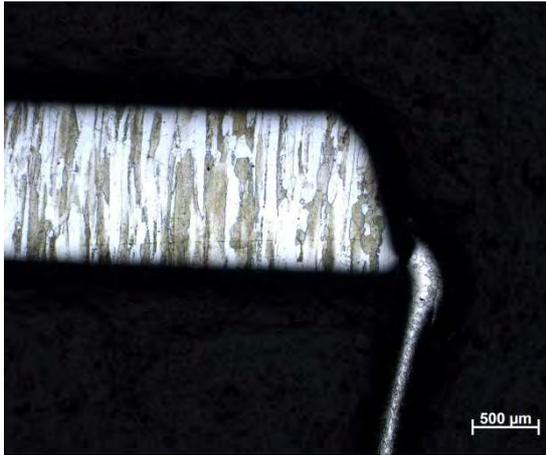
Fig.6. Evaporation and spattering of welded material in the case of a higher welding current  $SQ$  ( $TIME = 80$  ms;  $SQ = 50$  mA)
