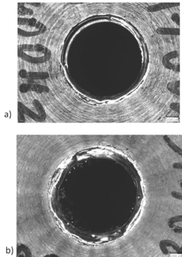
Fig.3. The macroscopic overview of a weld with the insufficient EB current SQ (a) – TIME = 80 ms, SQ = 35 mA) and with the adequate SQ (b) – TIME = 80 ms, SQ = 40 mA)
