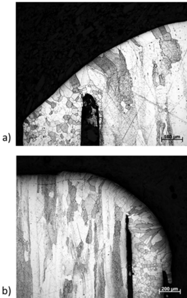
Fig.4. Example of the microstructure (LOM) of a weld for TIME = 80 ms, SQ = 40 mA (a) or for TIME = 80 ms, SQ = 45 mA (b)
