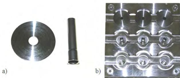
Fig.2. Parts of dummy testing sample (a) and sample mounted in welding fixture (b)
