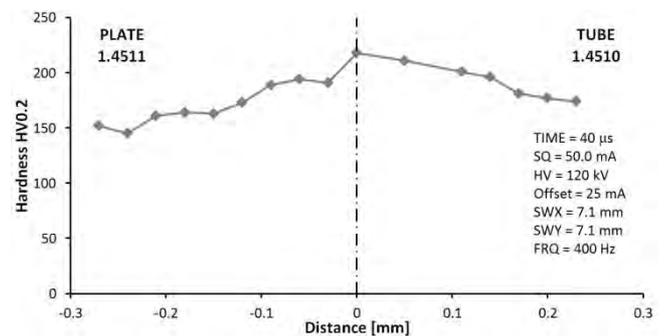
Fig.5. Example of hardness profiles HV0.2 measured in plate base materials through weld area to tube base material.
