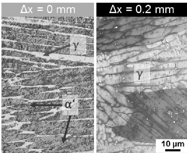
Fig. 3. The microstructure of the welding seam depended on the beam offset used.  $\gamma$ ...retained austenite;  $\alpha'$ ...Martensite
