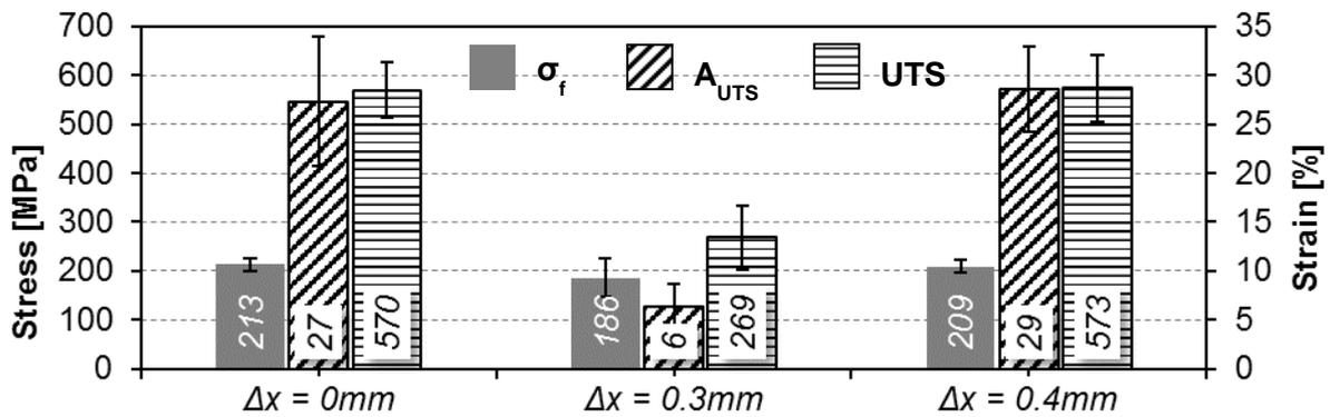
Fig. 7. Mechanical properties depended on the beam offset used
