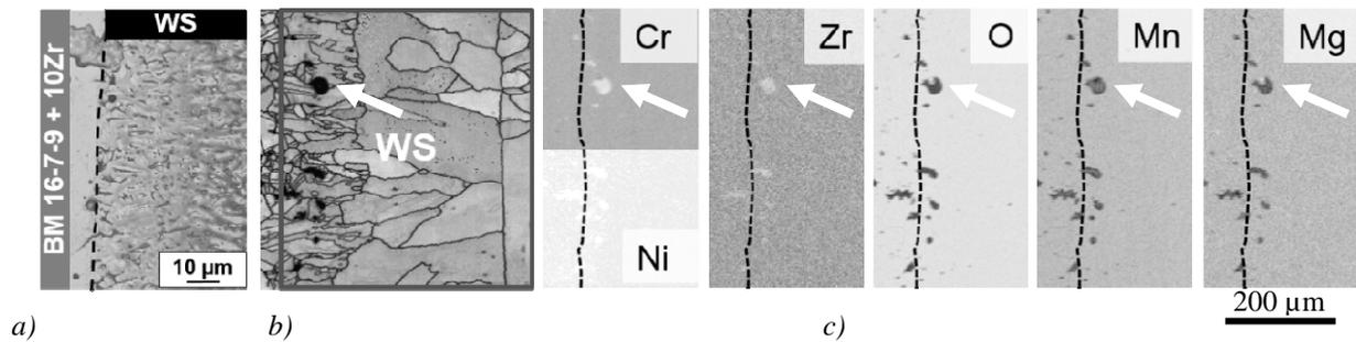
Fig. 9. EBSD measurements of the welded samples with  $D = 13\%$  and  $\Delta x = 0.3$  mm. a) light optical overview b) misorientation map with misorientation angle  $\theta$  (blue:  $15^\circ < \theta < 60^\circ$ , red:  $\theta = 60^\circ$ ), c) EDS mapping for different alloying elements. White arrows indicate positions of MnO/MgO.
