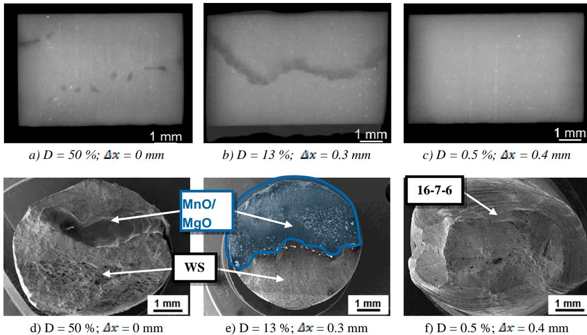
Fig. 8. a-c): Radiographs of longitudinal cross sections before tensile tests, d-f): fracture surfaces of the welded and tensile-tested samples after rupture
