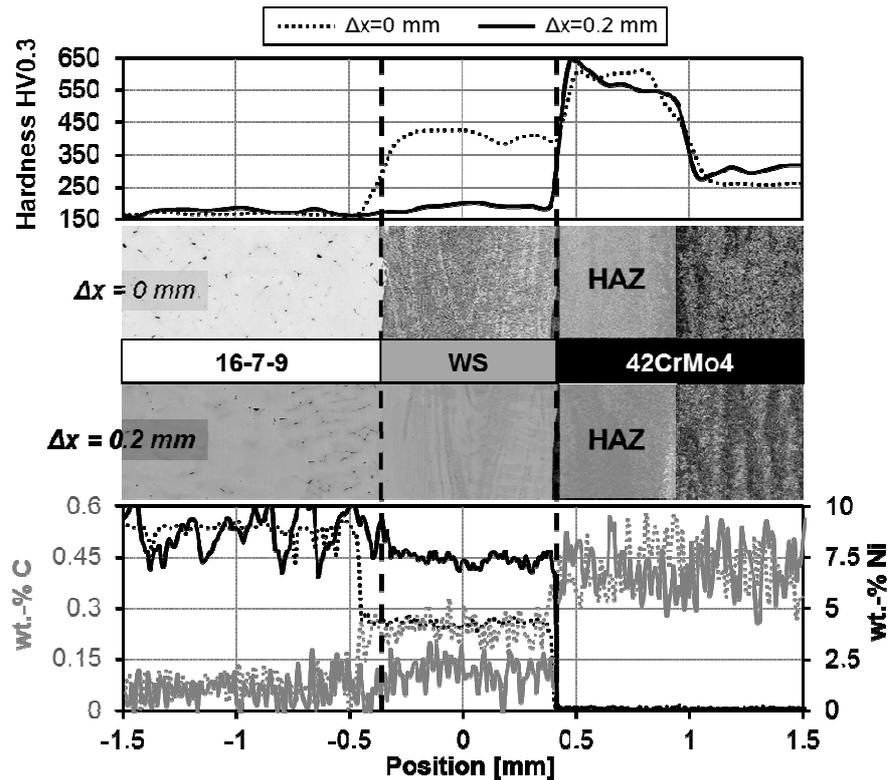
Fig.3. Micro-hardness profiles (top), macroscopic appearance (middle), and chemical composition according to WDS analysis (bottom) transverse to the welding direction as a function of the beam offset for a weld between 16-6-9 and 42CrMo4 steels.
