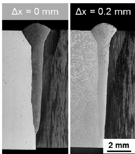
Fig. 2. The macroscopic appearance of the welding seam depending on the beam positioning relative to the welding gap (welding partners: 16-7-9 + 42CrMo<sub>4</sub>)
