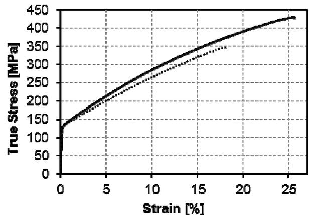
Fig. 4. Representative true stress-strain curves depended on the beam offset used
