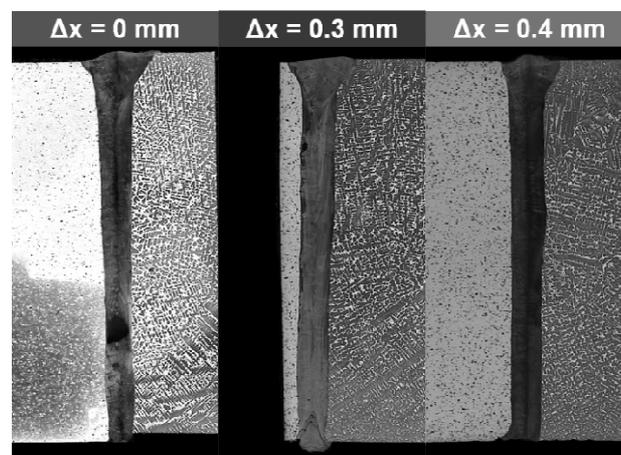
Fig. 6. Macrographs of the welded butt joints as a function of the beam offset used. White arrows indicate the location of pores/cavities
