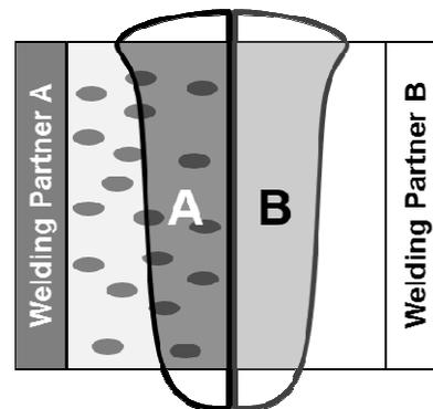
Fig. 1. Schematic diagram for the quantification of the dilution
