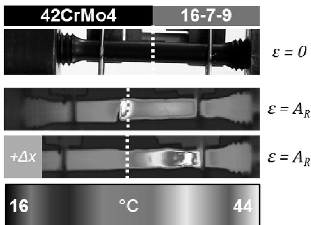
Fig. 5. Macroscopic appearance of the tested samples ( $\epsilon = 0$ ) and temperature distribution at rupture ( $\epsilon = A_R$ ) for different beam offsets. Dashed line: welding seam
