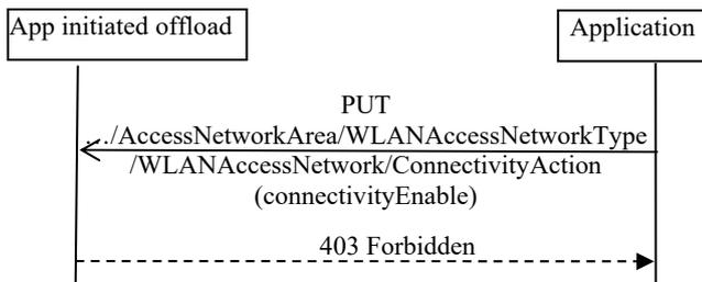
Fig.4 Unsuccessful application-initiated offloading to WLAN.
