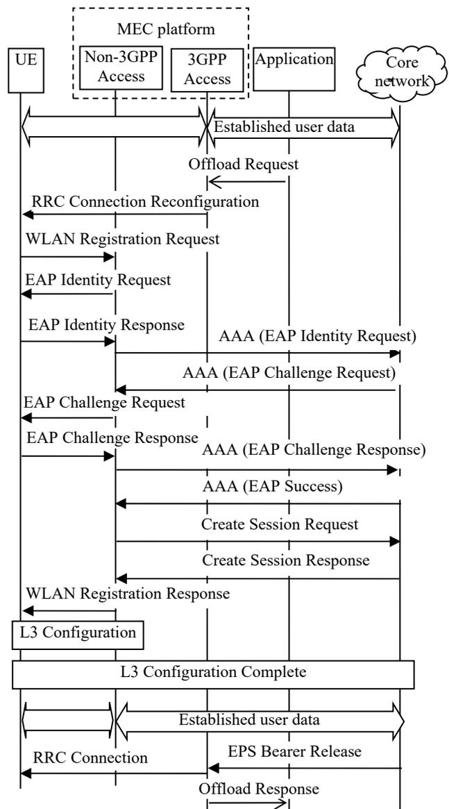
Fig.1. Mobile edge application initiated handover from 3GPP access to trusted WLAN.
