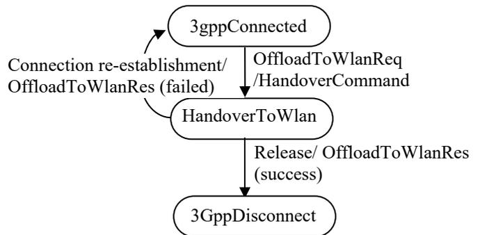
Fig.6 Offloading state model as seen by the serving 3GPP access network.
