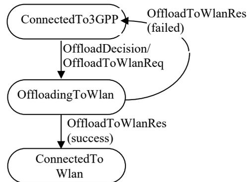
Fig.5 Application view on the offloading state.
