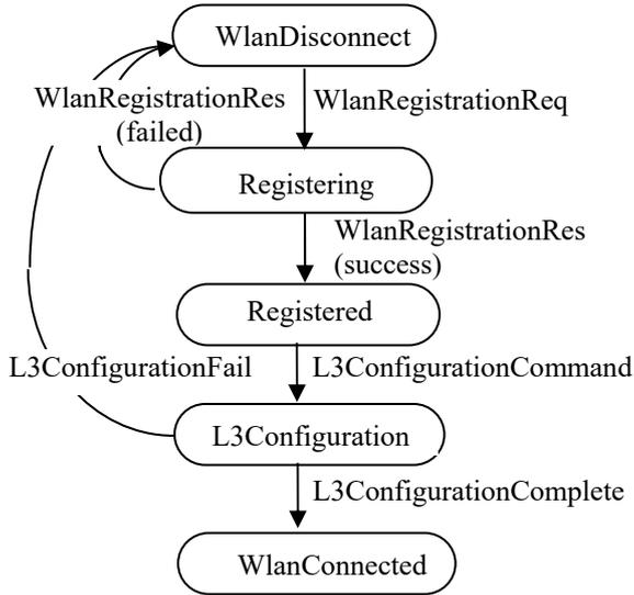
Fig.7 Offloading state model as seen by the target WLAN.
