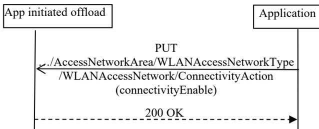
Fig.3 Successful application-initiated offloading to WLAN.
