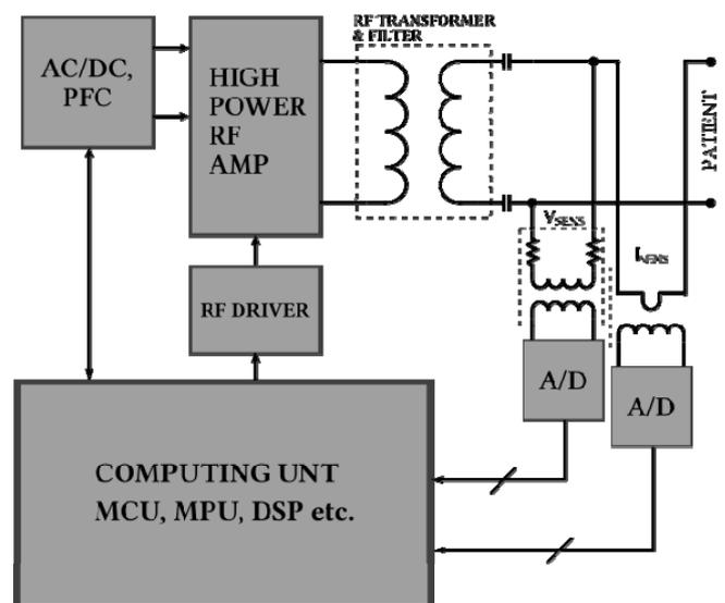
Fig.3. Simplified block diagram of a closed loop scheme.
