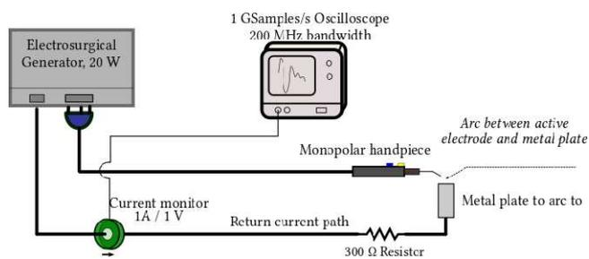
Fig.4. Experimental setup to investigate the current waveform in spark conditions.
