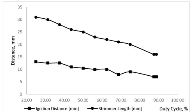
Fig. 7. Ignition distance and strimmer length depending on the duty cycle.
