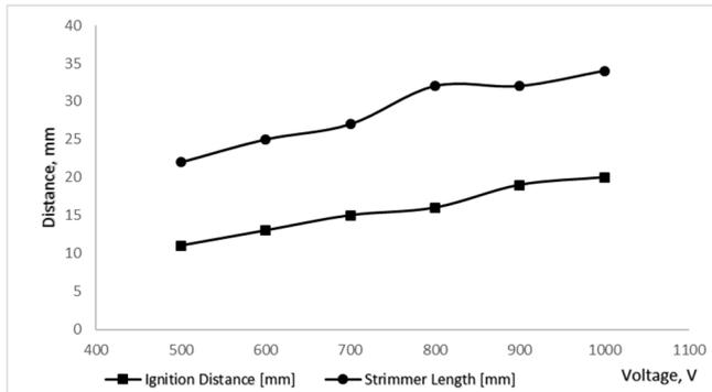
Fig. 5. Ignition distance and strimmer length depending on the maximum output RMS voltage.
