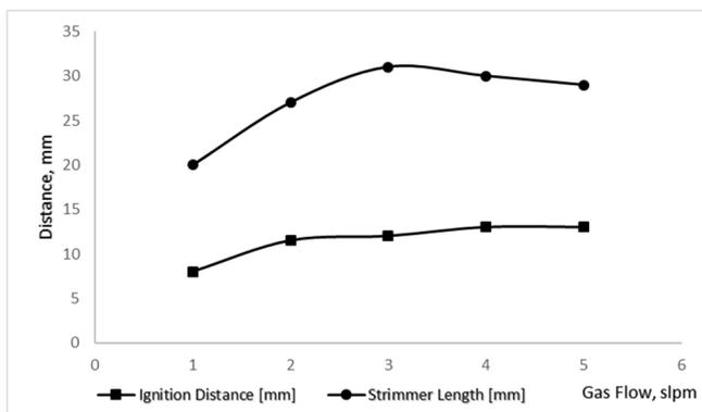
Fig. 6. Ignition distance and strimmer length depending on the gas flow rate.
