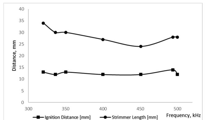
Fig. 12. Ignition distance and strimmer length depending on the frequency at  $V_{RMS}$  700V.
