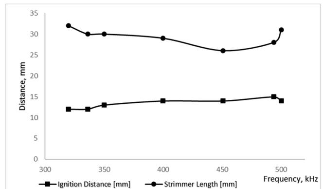
Fig. 11. Ignition distance and strimmer length depending on the frequency at  $V_{PP}$  5kV.
