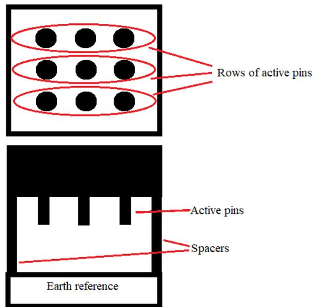
*Fig. 1. Example structure for Plasma based sterilization accessory.*
