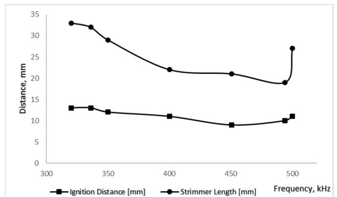
Fig. 8. Ignition distance and strimmer length depending on the output signal frequency.
