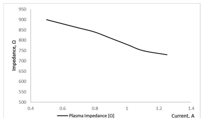
Fig. 4. Plasma impedance depending on the maximum output RMS current.
