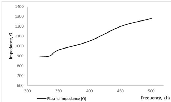
Fig. 9. Impedance of the plasma depending on the output signal frequency.
