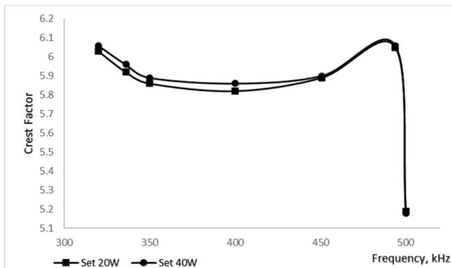
Fig. 10. Calculated CF (crest factor) of the output signal depending on the frequency.
