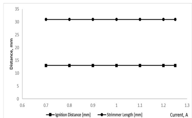
Fig. 3. Ignition distance and strimmer length depending on the maximum output RMS current.
