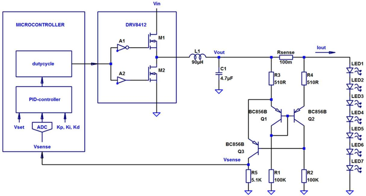
Fig. 1. Schematic of the proposed digital PID-controller for LED applications.
