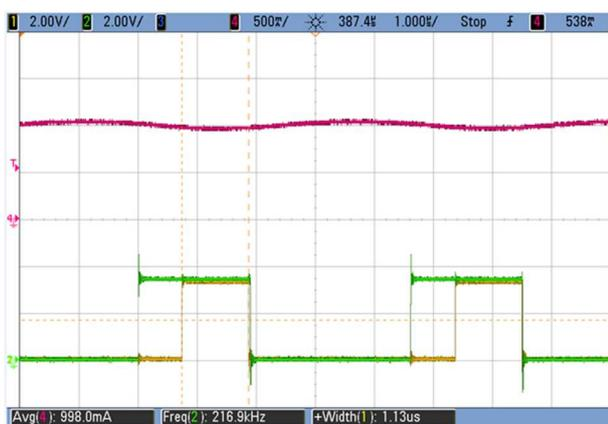
Fig.4. Steady state operation of the LED driver (red – LED current, yellow – PID controller execution time, green – PID controller output PWM).
