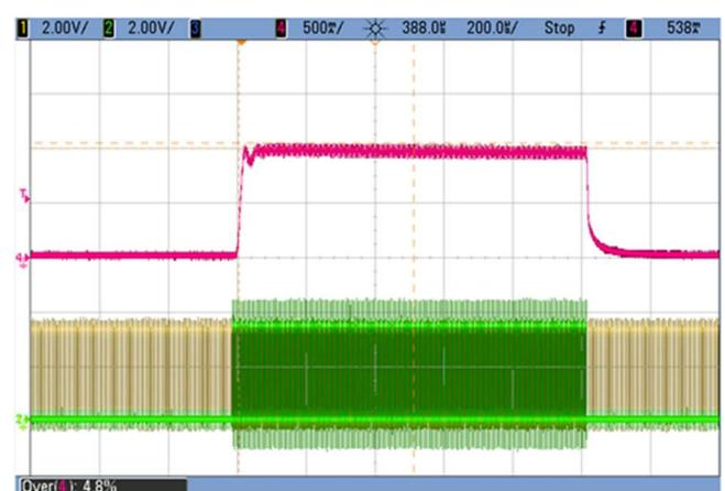
Fig.5. LED current overshoot tuning (red - LED current).
