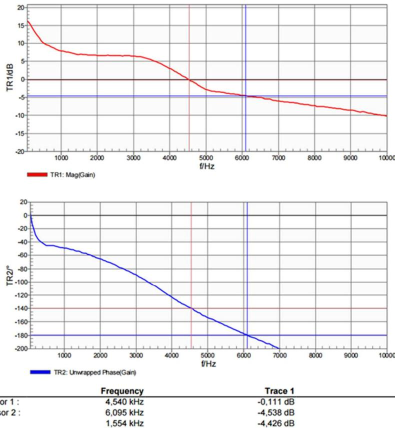
*Fig.8. Bode plot of the tuned LED driver.*
