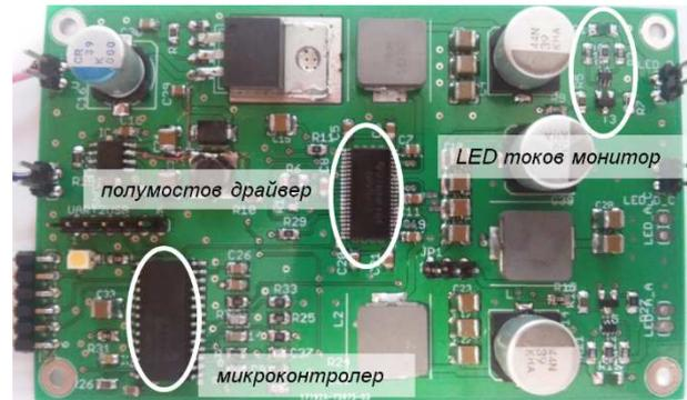
Fig.3. Prototype PCB, top view.
