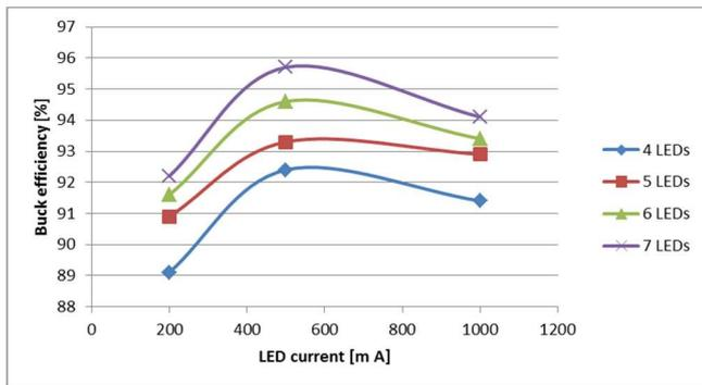
Fig.9. Efficiency plot of the tuned LED driver.
