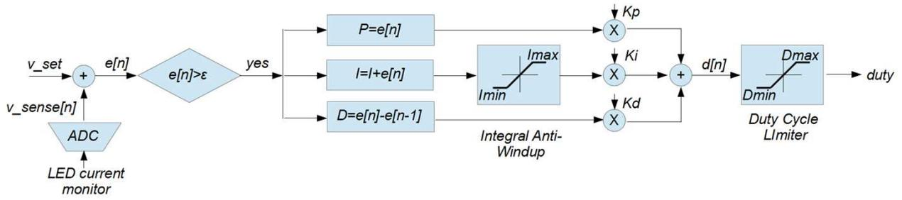
Fig.2. Block diagram of the digital PID controller with anti-windup algorithm.
