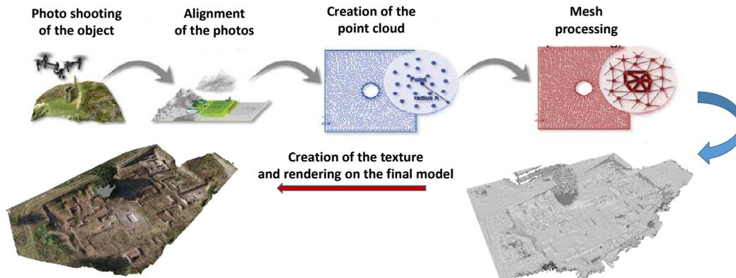
Fig. 1. Processing the digitalized data and creation of the 3D model.
