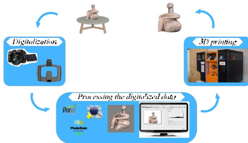
Fig. 2. The complete process for 3D reconstruction of a small object
